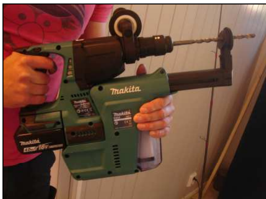
Figure 10-19. Drill for Surface Samples
