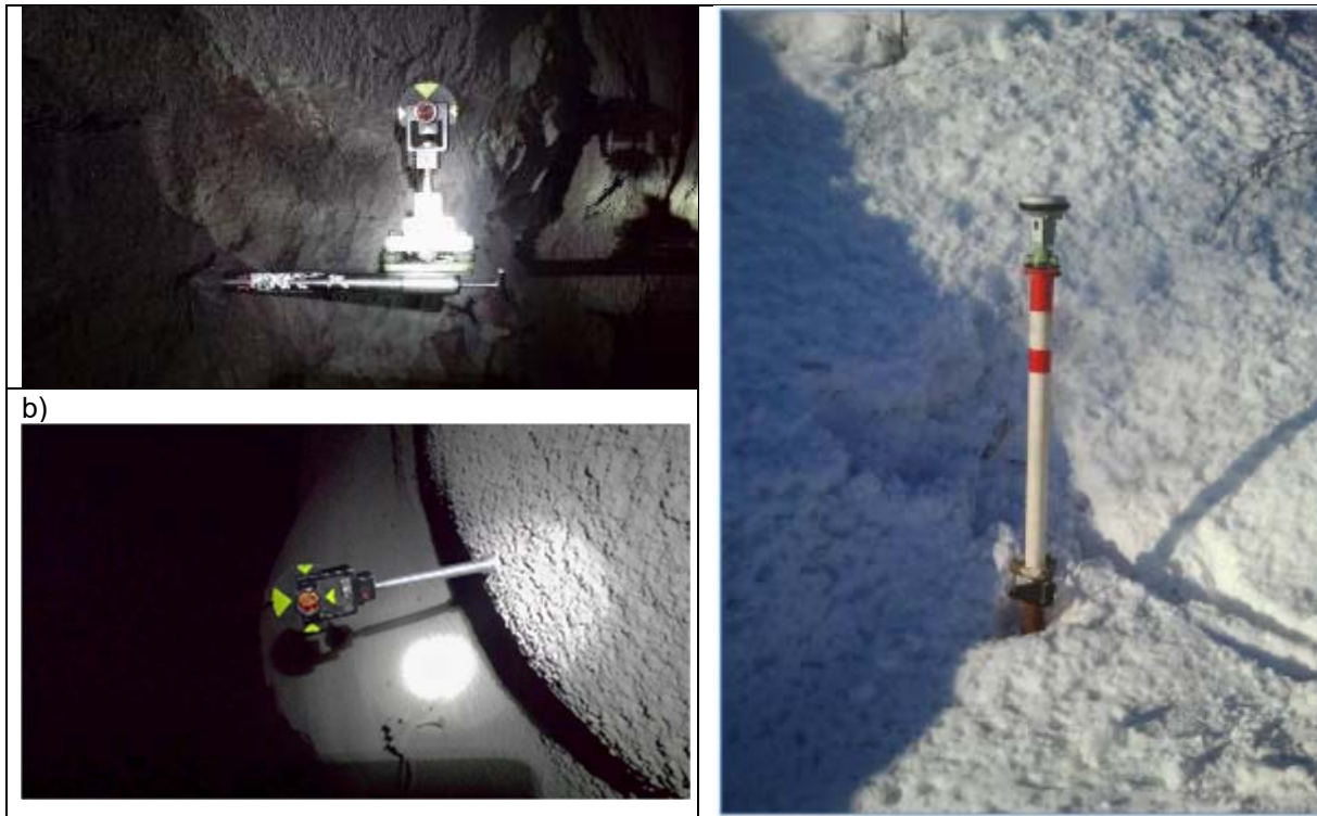
Figure 1-40: a) Permanent control station in tunnel wall. b) Short term control station using a bolt in the wall. c) Control station mounted on a pole outside the mine entrance.
