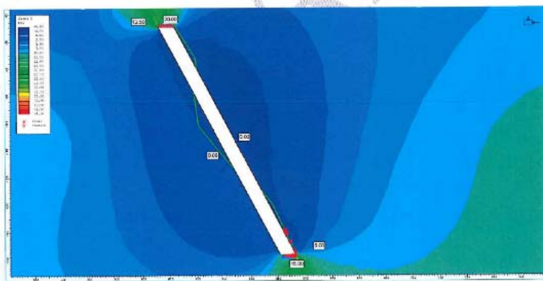
Figure 1-18: Model#4 - Vertical stress and yielded zone for Stope D (SINTEF, 2016c)
