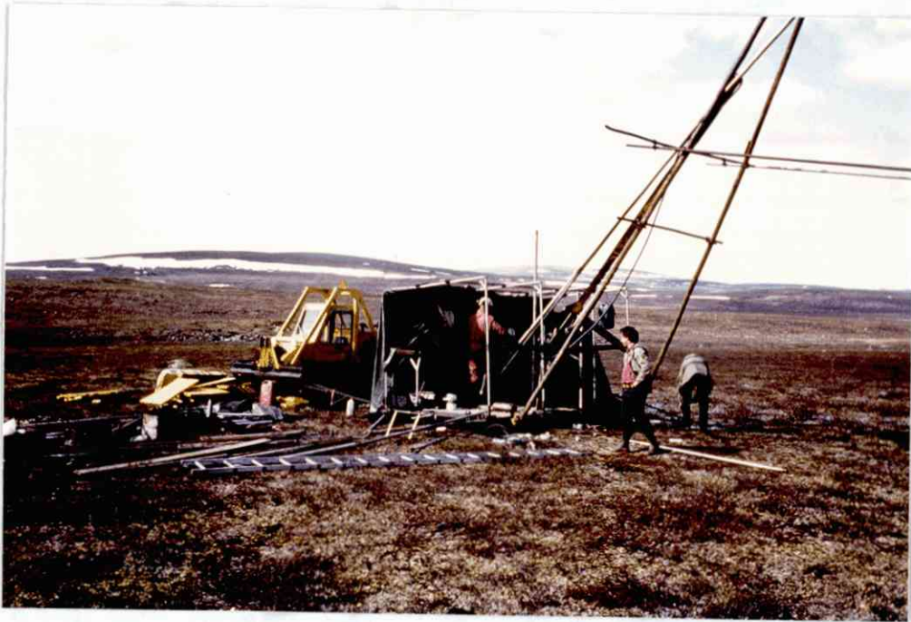
Fig. 3. Diamond drill hole 140 D was drilled with ASPRO's Longyear 24 drill.
