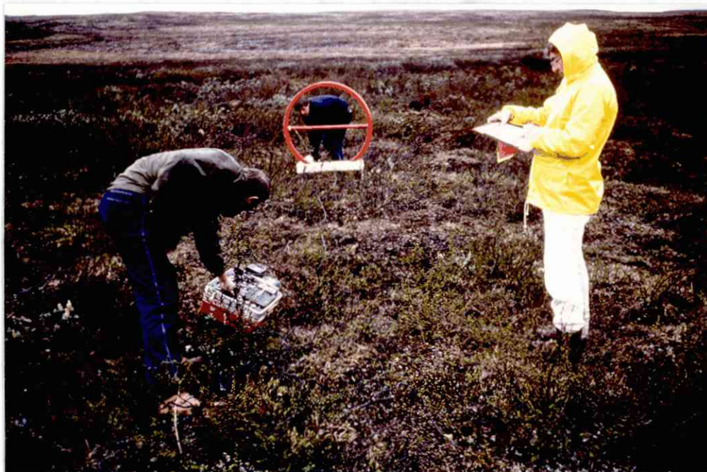
Fig. 5. EM-37 test survey in Bidjovagge. Receiver with receiver coil in position to measure the horizontal field component.
