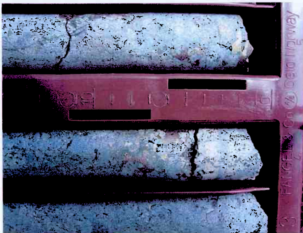
Photo 10.2d: View of Bjørndalsnipa core with interstitial chalcopyrite and pyrrhotite
