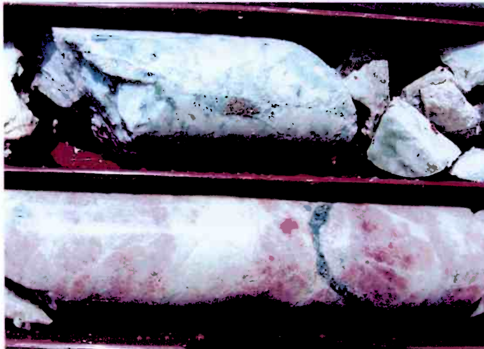
Photo 10.2e: View of BJN-8 core with interstitial pyrrhotite.
