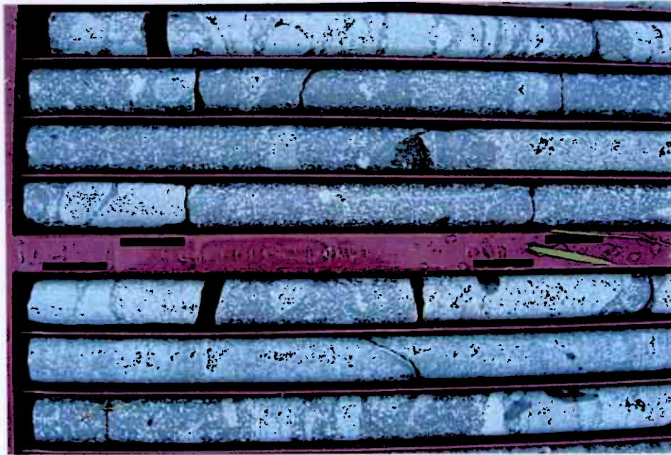
Photo 10.1b: View of HGV-2 core showing heterolithic "cobbles" of anorthosite in a massive to disseminated ilmenite matrix
