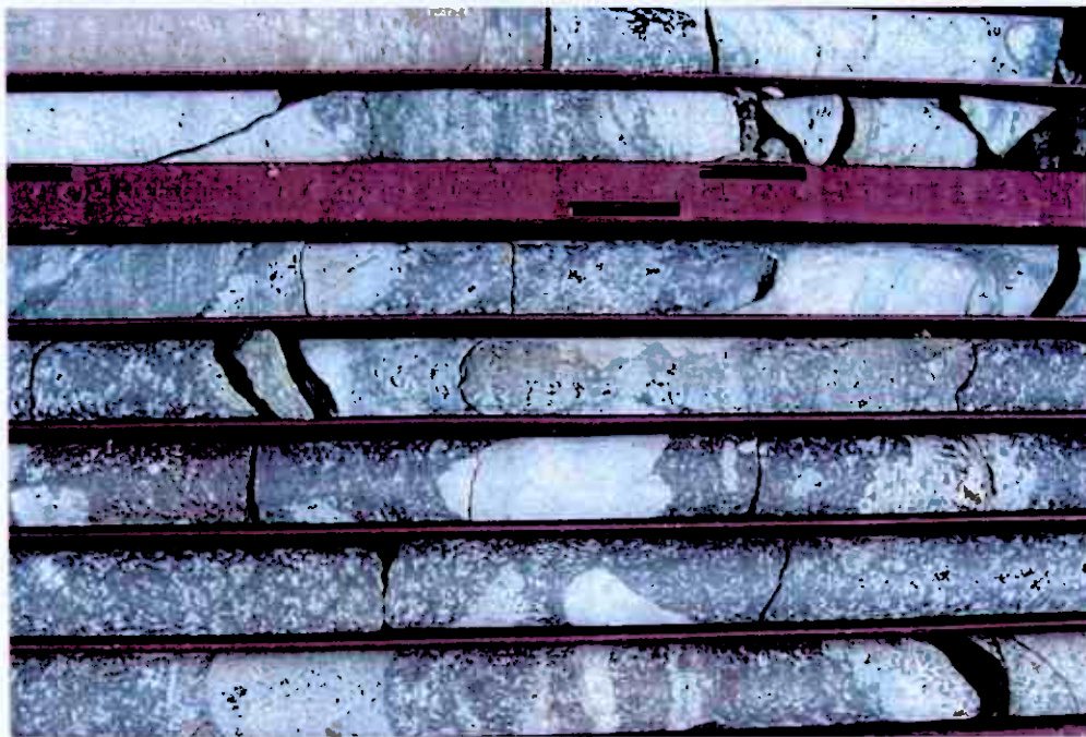
Photo 10.1c View of HGV-2 core showing heterolithic "cobbles" of anorthosite in a massive to disseminated ilmenite matrix
