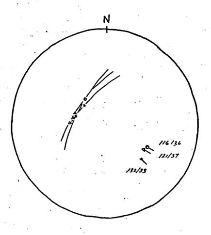
Fig. 5 Orientation of the flanks of the ore controlling fold structures at Knaben I and II and  $\emptyset$ rnehommen. The foldaxes are constructed.
