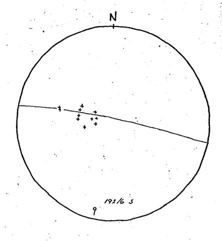
Fig. 2 Foliation measurements and constructed foldaxis from the area between Reinshommen and Knaben I.
