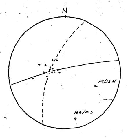
Fig. 4 Foliation measurements and constructed foldaxes from the area around Kvina.
