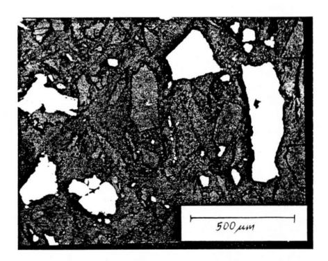
Photomicrograph of -300  $\mu m$  fraction  $(White \ grains \ - \ arsenopyrite, \ dark \ grains \ - \ gangue \ material)$
