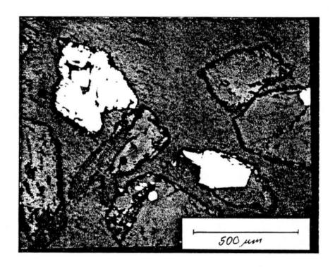
Photomicrograph of -600+300  $\mu m$  fraction  $(White\ grains\ -\ arsenopyrite,\ dark\ grains\ -\ gangue\ material)$
