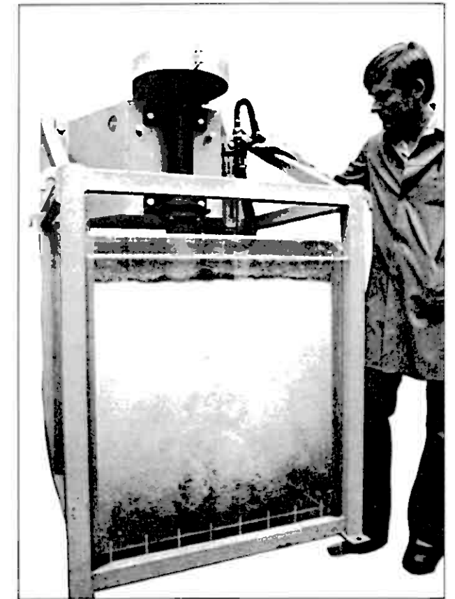
Studying basic features of air dispersion and pulp agitation in a 500 litres flotation cell.
