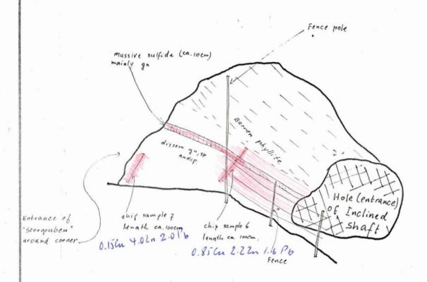
Sketch of cliff wall between "Storgruben" and entrance to Inclined Shaft.
