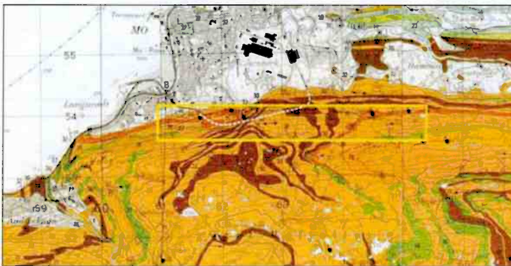
Figure 1: Geological map of the Mofjellet mining area. The railway tunnel is marked with a white stippled line. The yellow line shows the extent of the mined ore body. Orange, yellow and green colours are various gneisses, and brown is amphibolites.
