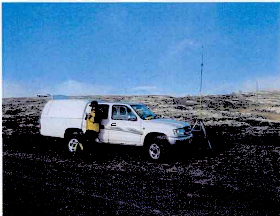
Figure 4.3.1 GPS Repeater set up next to road
