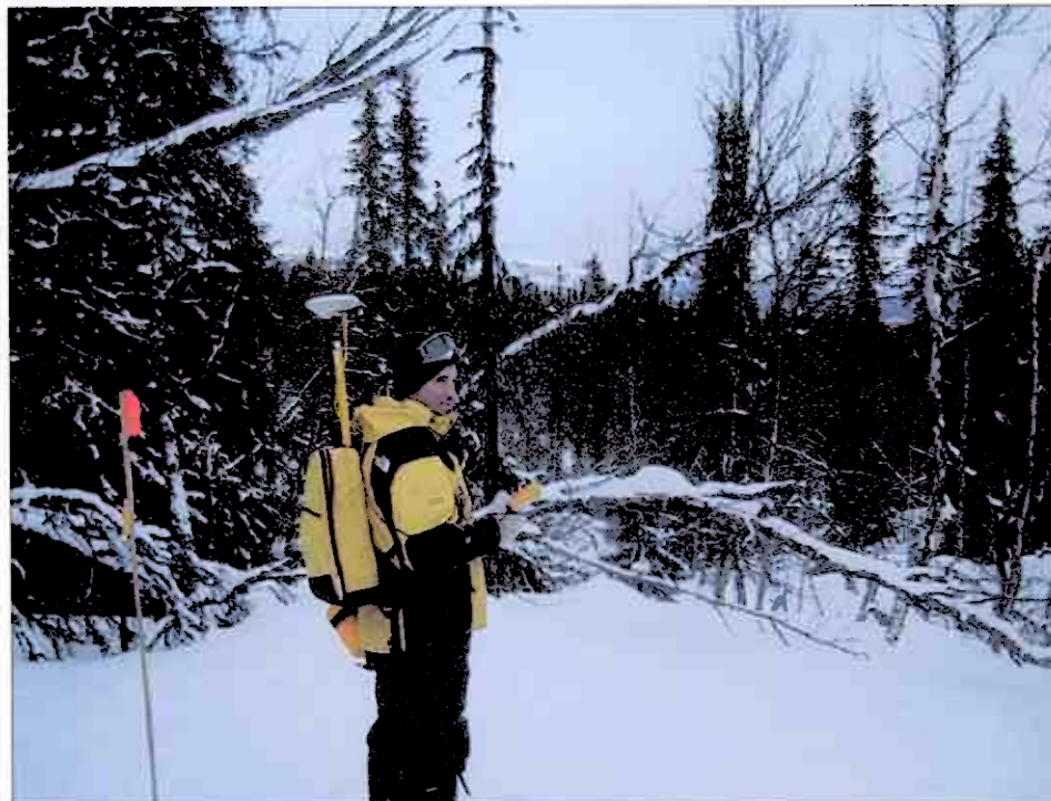
Figure 4.3.1 The author wearing Trimble GPS backpack
