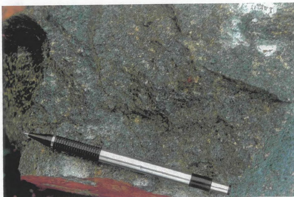
Photograph 2.1 – Disseminated pyrite-chalcopyrite in metapyroxenite
