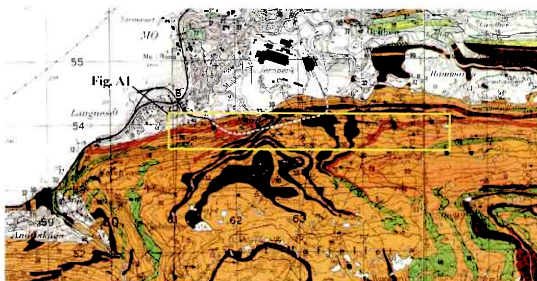
Figure 1: Bedrock map of the Mofjellet mining area. The railway tunnel is marked with a white stippled line. The frame of Fig. A1 (yellow line), shows the extent of the mined ore body. Orange, yellow and green colours are various gneisses, and brown is amphibolites. For detailed legend of the bedrock, see Sovegarto et al. (1988). Note the favourable location of the mining area close to harbour and the city of Mo i Rana. The grid is 1 x 1 km.
