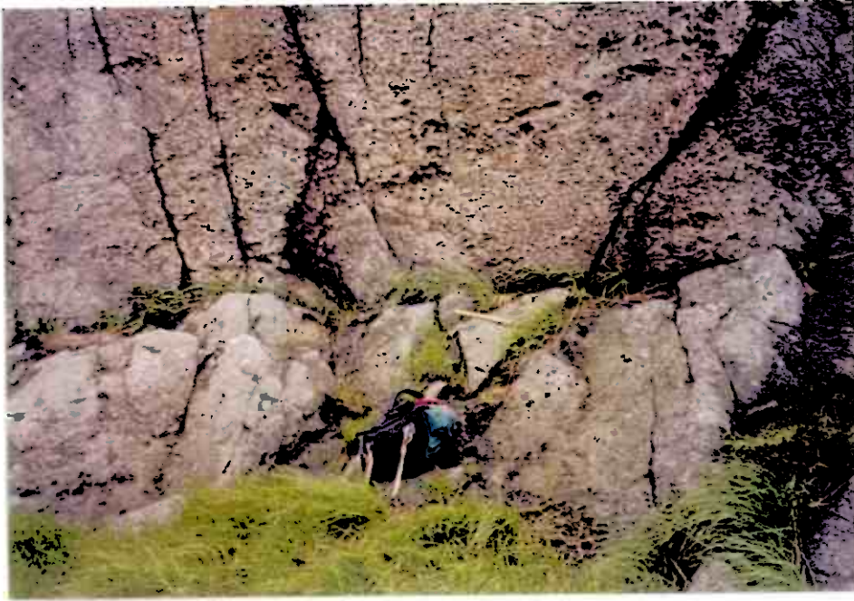
Contact between anorthosite (bottom) and coarse norite west of Sulfidmalm's drill holes. The norite truncates the anorthosite and is the reason that the conductive zone does not crop out. The HEM conductor is about 25 meters below the backpack.
