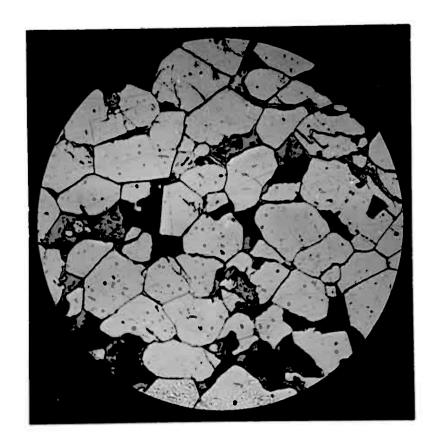
Plate 14, Fig. 1. Fyrite (white) being replaced by sphalerite (gray). Reflected light. X 200.
