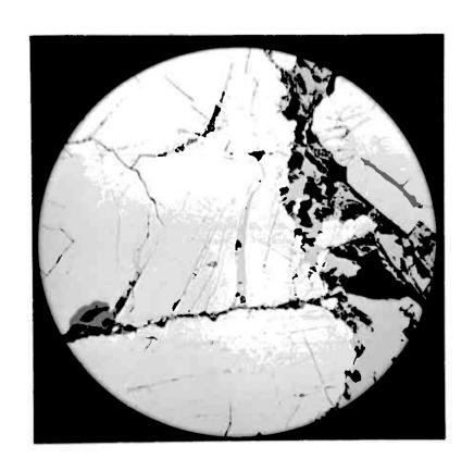
Plate 12, Fig.1. Tyrite cube (white) penetrated by a silicate gangue mineral (black). Reflected light. X 200.
