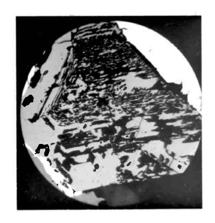
Plate 5, Fig. 1. Massive pyrite ore folded into quartzitic schists of the foot wall. Daylight.
