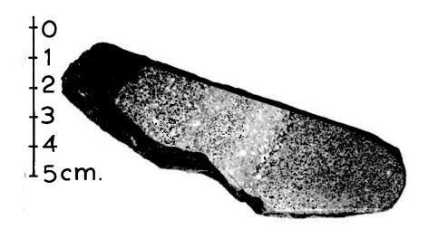
Plate 10, Fig. 1. Enlargement of Flate 8, Fig. 2 showing detail of banded pyrite ore. Daylight.
