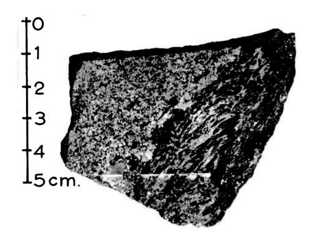
Plate 7, Fig. 1. Nagnetite (black) banded pyrite ore (white) showing typical lensing of the magnetite. Daylight.
