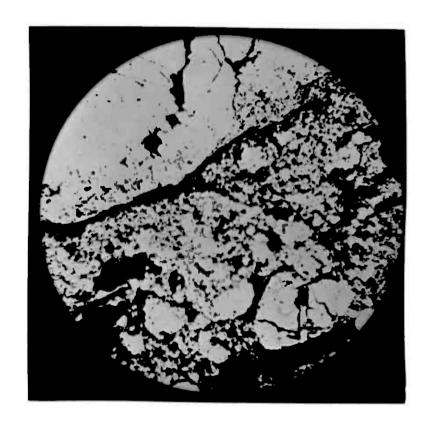
Plate 4, Fig. 1. Etched pyrite crystal (white) mounted in plastic (gray) showing an embayment which in polished section appears to be an inclusion. Reflected light. X 200.
