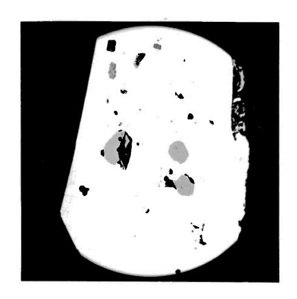
Plate 12, Fig. 1. Fine-grained dusty pyrite (white) with sphalerite (gray). Reflected light. X 200.
