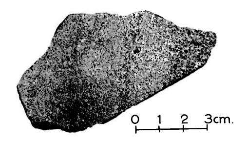
Plate 8, Fig. 1. Massive pyrite ore banded by change in grain size in contact with undifferentiated schists. Daylight.
