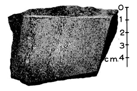
Plate 9, Fig. 1. Massive pyrite ore with band of coarse pyrite crystals. Daylight.
