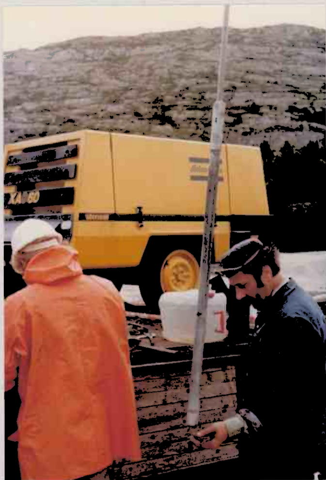
Fig. 6 The 1 m long iron-tube used for sampling the tailing
