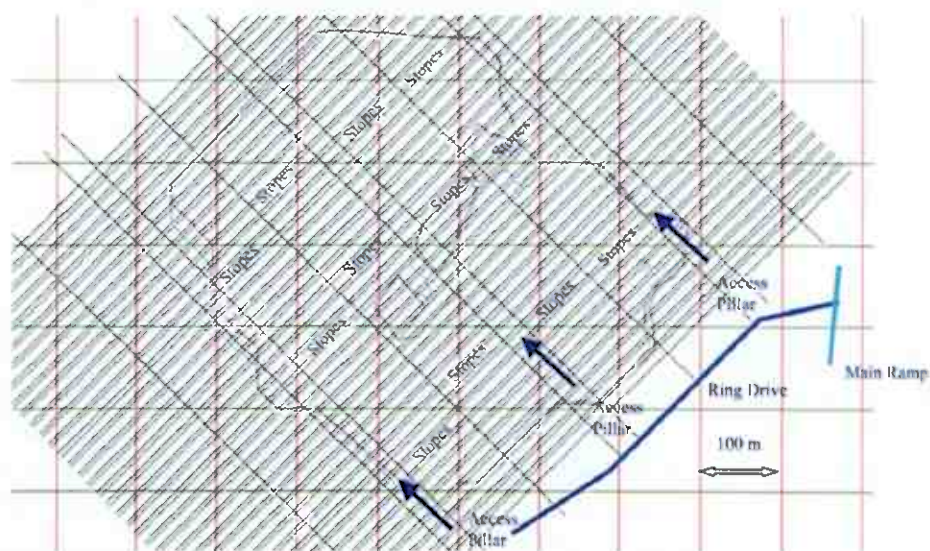
Figure 16 – Primary mining with pillars between mining blocks and the stopes
