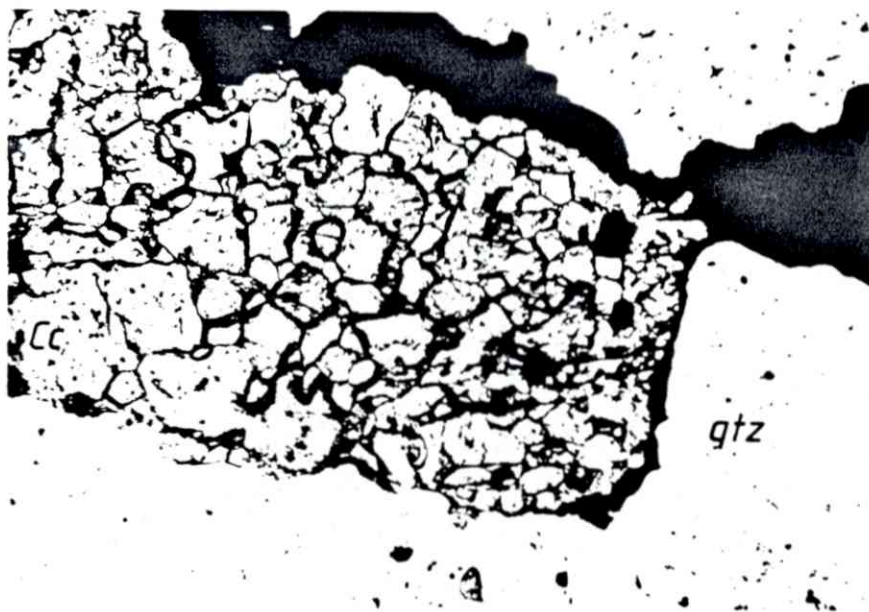
fig. 13: 8 0 0 1 0 4, banded remobilized calcareous gneiss, // nicols, thin section, magnification x 63, vein-type like mobilization of calcite, quartz and sulfides.
