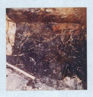
FIGURE 12. UNDERGROUND EXPOSURE OF MICA-RICH BASIC SILICATE ROCK (UNIT C). THE IRREGULAR NETWORK OF WHITE CALCITE SEGREGATIONS AND VEINS OF SØVITE TYPIFY THIS ROCK UNIT. A RECTANGULAR PORTION OF A DIKE OF RAUHAUGITE (UNIT G) IS SHOWN ON THE LEFT. PHOTO NO. 0020-3; NEAREST GRID INTERSECTION IS 142.020 - 51.280.
