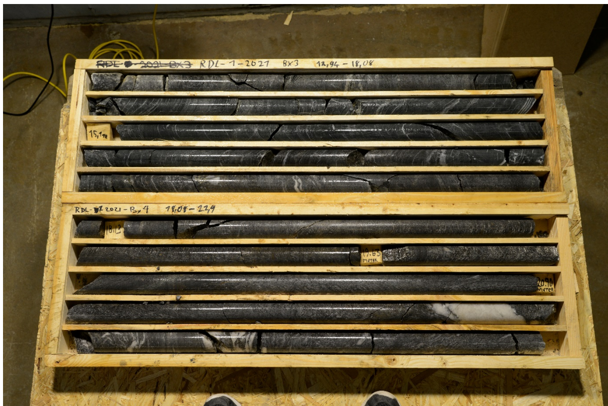
Figure 5: Rødalen hole 1 box 3 and 4 13 to 23m showing amphibole layer between 13.8 and 17.2m
