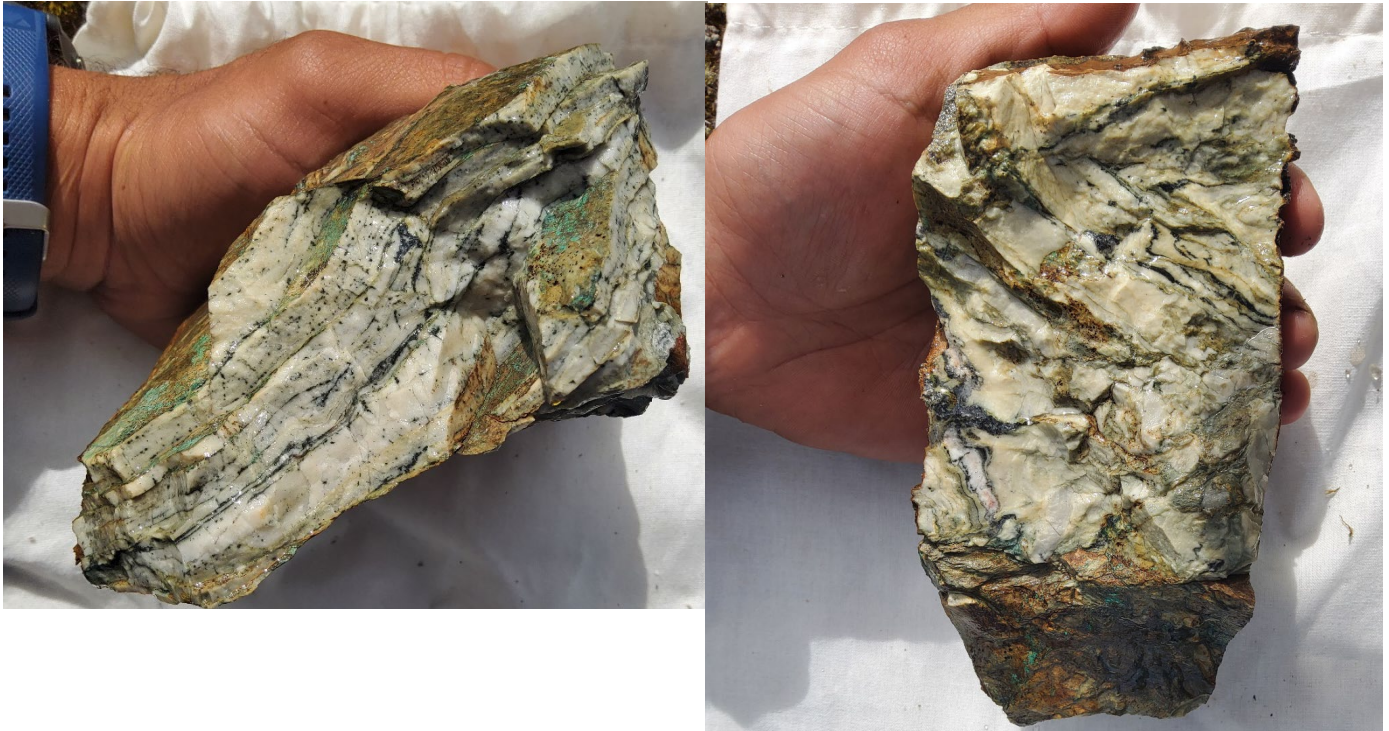
Figure 8 - Main outcrop rock samples. White/cream coloured dolomite with disseminated chalcocite along fine layers. Malachite staining on planes. Rare bornite visible.
