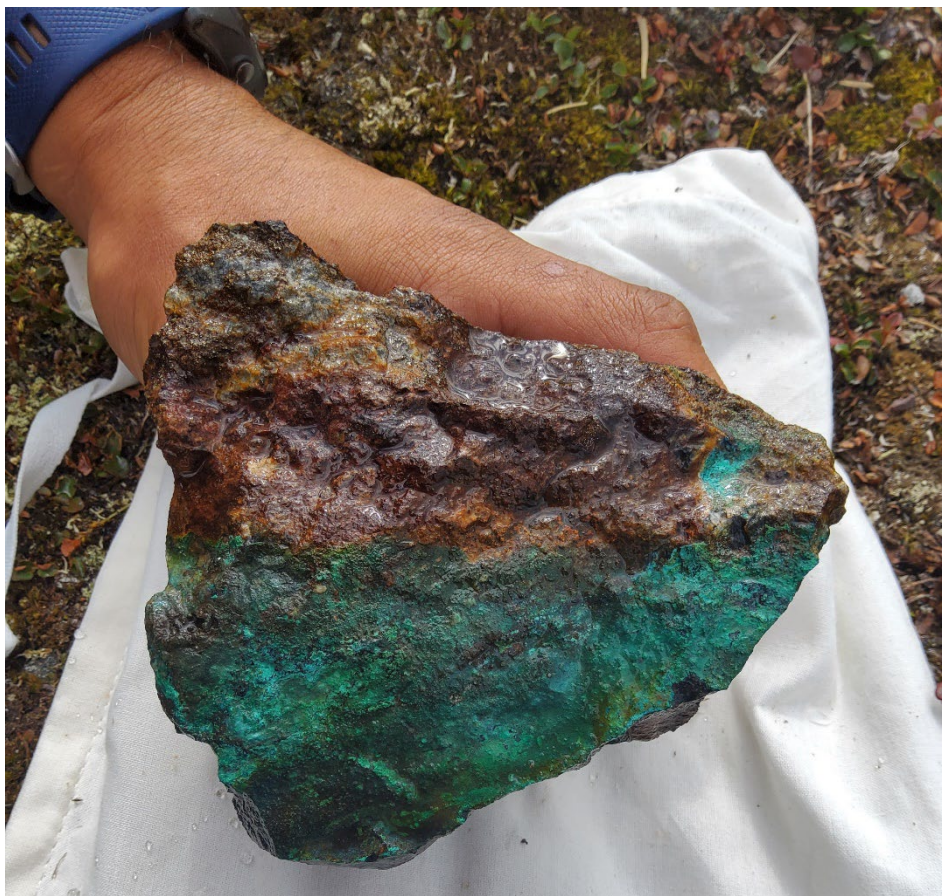
Figure 7 - Antler Rock outcrop sample showing secondary copper mineralisation.
