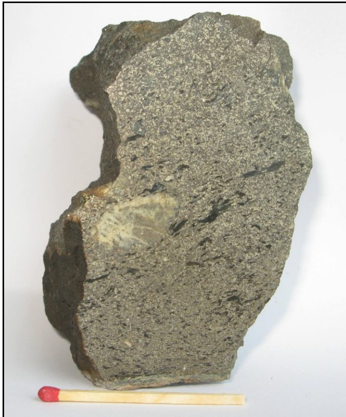
Figure 9: Tjo5, massive sphalerite and pyrite with traces of chalcopyrite and possibly galena. Matrix is quartz and minor chlorite. The sample is not analysed but has in excess of 20% zinc.
