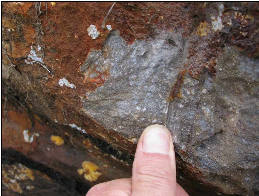
Figure 13: Massive sphalerite with rounded fragments of silicates at Tjo7. Fragments of this layer went into sample 563524 together with fragments from the less zinc-rich sulphide layer depicted on the frontpage. It would have been better with two separate samples.
