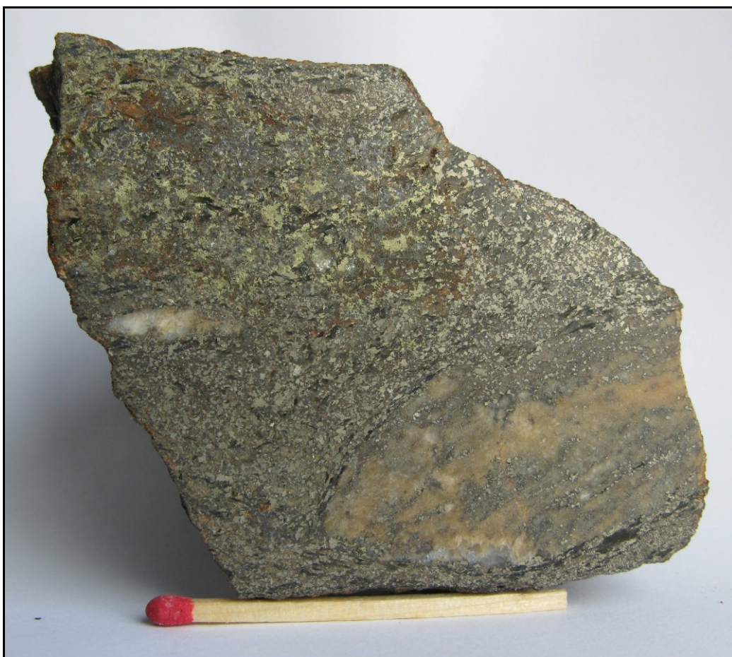
Figure 10: Tjo5, sample 563405. Massive chalcopyrite, pyrite and sphalerite in quartz matrix. 6.4 ppm gold, 74 ppm silver, 4.9% copper, 9.9% zinc and 0.4% lead.
