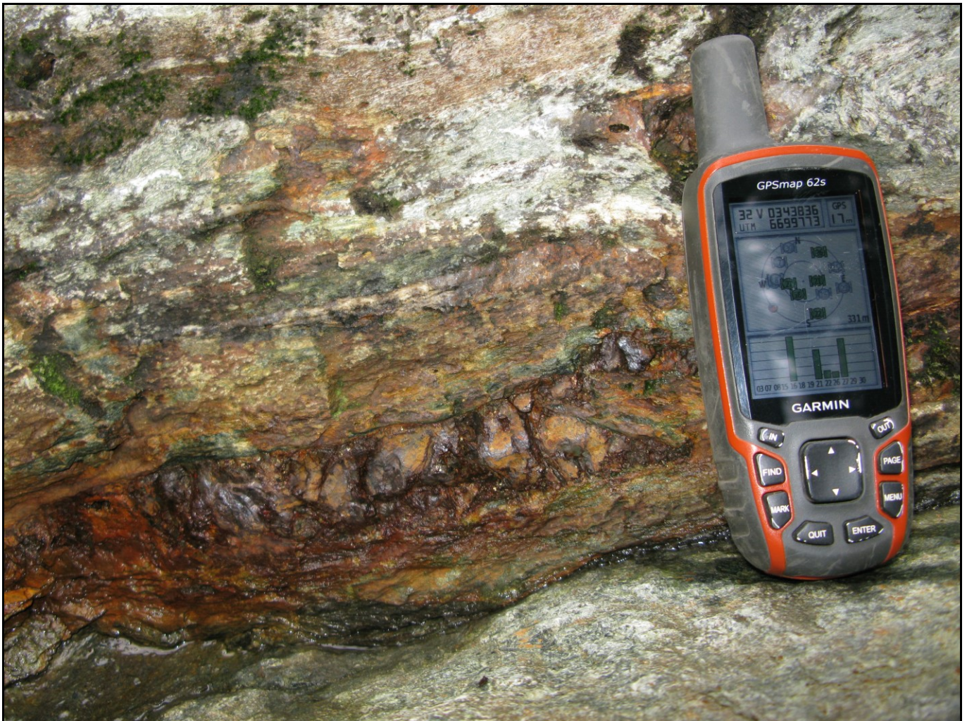
Figure 22: One of the four-five coarse-grained massive pyrrhotite>>chalcopyrite layers at Tjo19. Sample 563540 is made up of fragments from this layer and the outcrop's other sulphide layers. These massive sulphide layers are not traditional VHMS-style.
