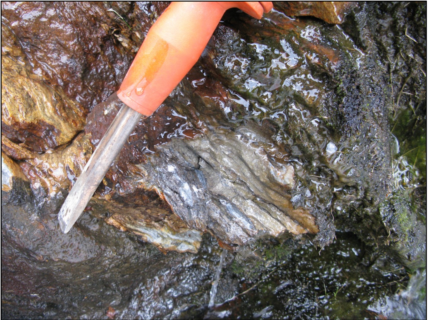
Tjosås, one of the two massive sulphide layers at Tjo7. The upper part is mostly pyrite while the lower is high in sphalerite.
