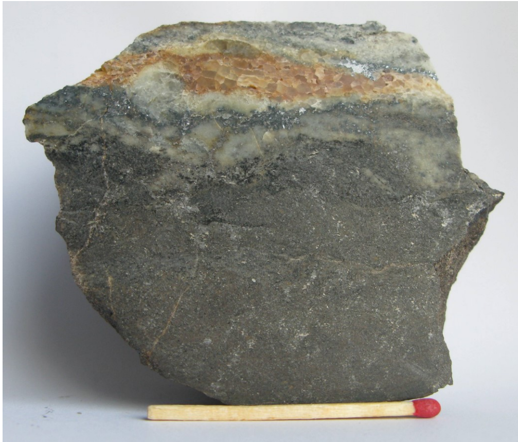
Fig. 2.4.2: Espelandsmyr, sample 563335. Lower part is fine-grained quartz and biotite with weak dissemination of galena and sphalerite. Upper part is quartz with galena, sphalerite and possibly traces of pyrrhotite.
