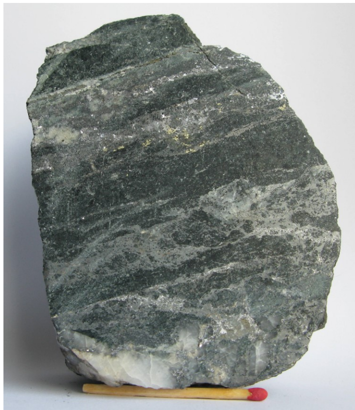
Fig. 2.6.3: Skolteberg, sample 563341. Chloritized metabasalt (?) with bands of galena, sphalerite and minor chalcopyrite.
