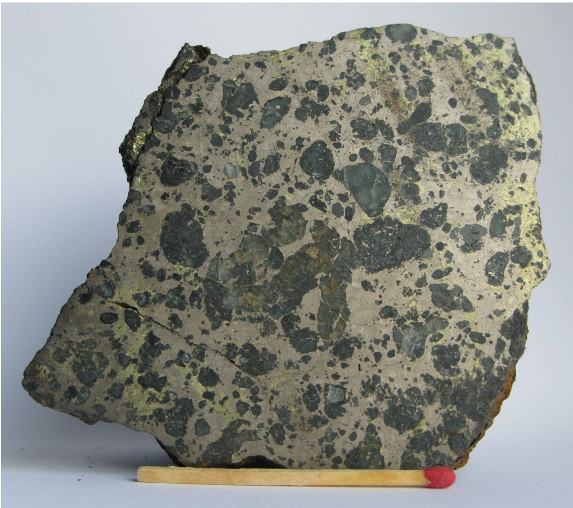
Fig. 2.5.3: Rørholt, sample 563339. Textbook example of ball-texture. Rounded quartz clasts in matrix of pyrrhotite and chalcopyrite.
