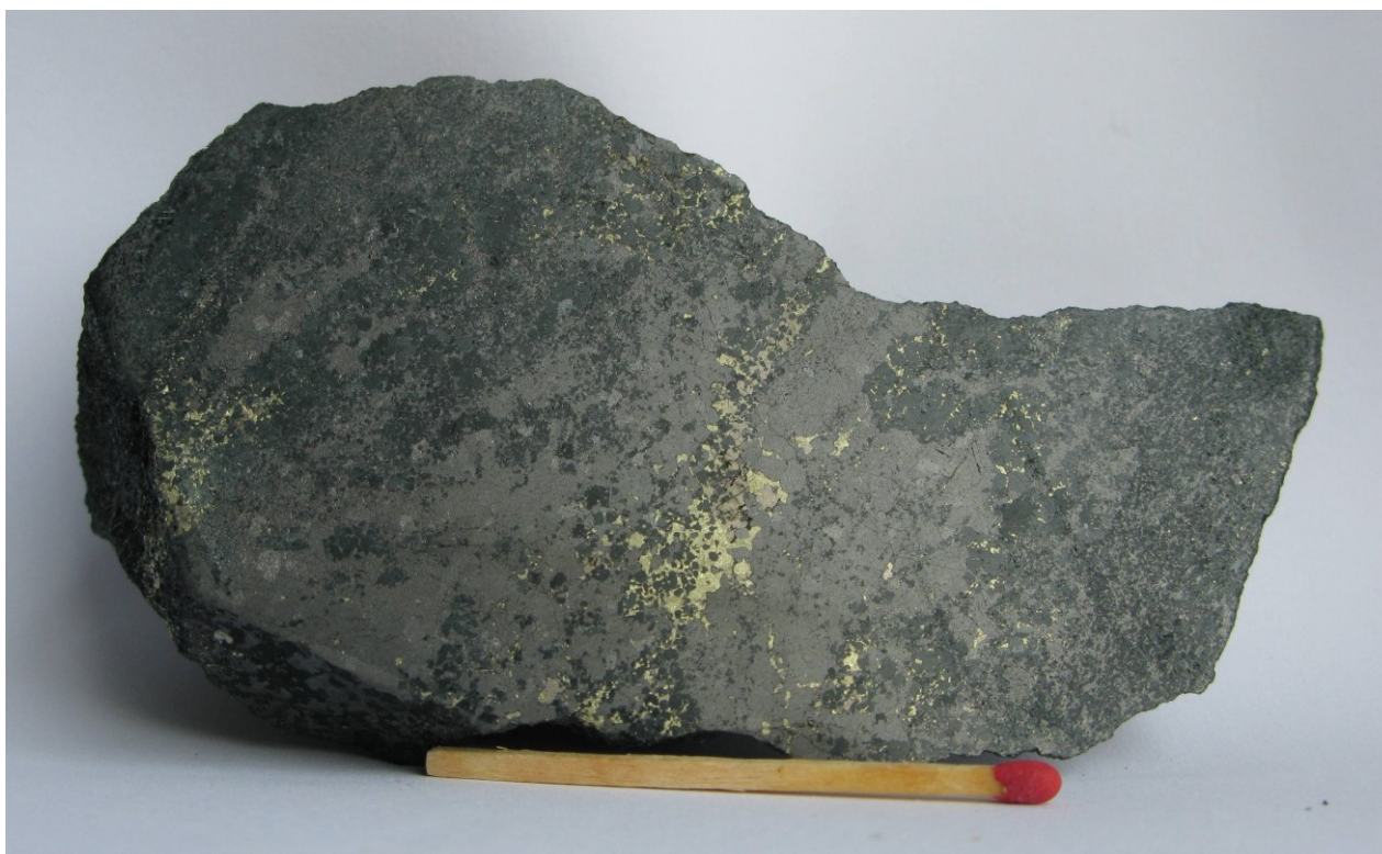
Fig. 2.17.2: Haugset, sample 563361. Amphibole and magnetite with chalcopyrite and minor pyrite. Although not evident in this cut, the sulphides occur in bands in this type of ore.
