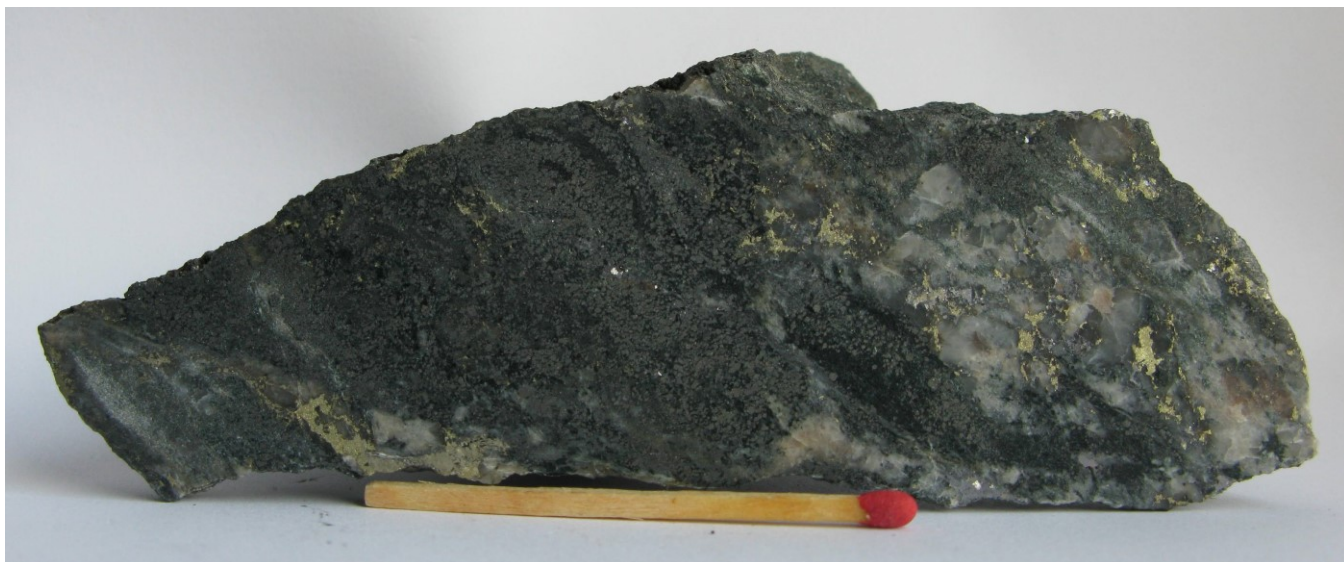
Fig. 2.6.4: Skolteberg, sample 563342. The most copper- and gold-rich specimen found. Tectonized quartz and chlorite with magnetite (left half) and chalcopyrite, sphalerite and pyrite.
