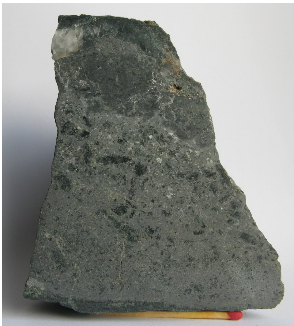
Fig. 2.7.3: Gunhildskås 1, sample 563364. Fine-grained ore breccia with galena, sphalerite and minor chalcopyrite and magnetite. Rounded clasts (ball texture) are quartz and chloritized metabasalt.
