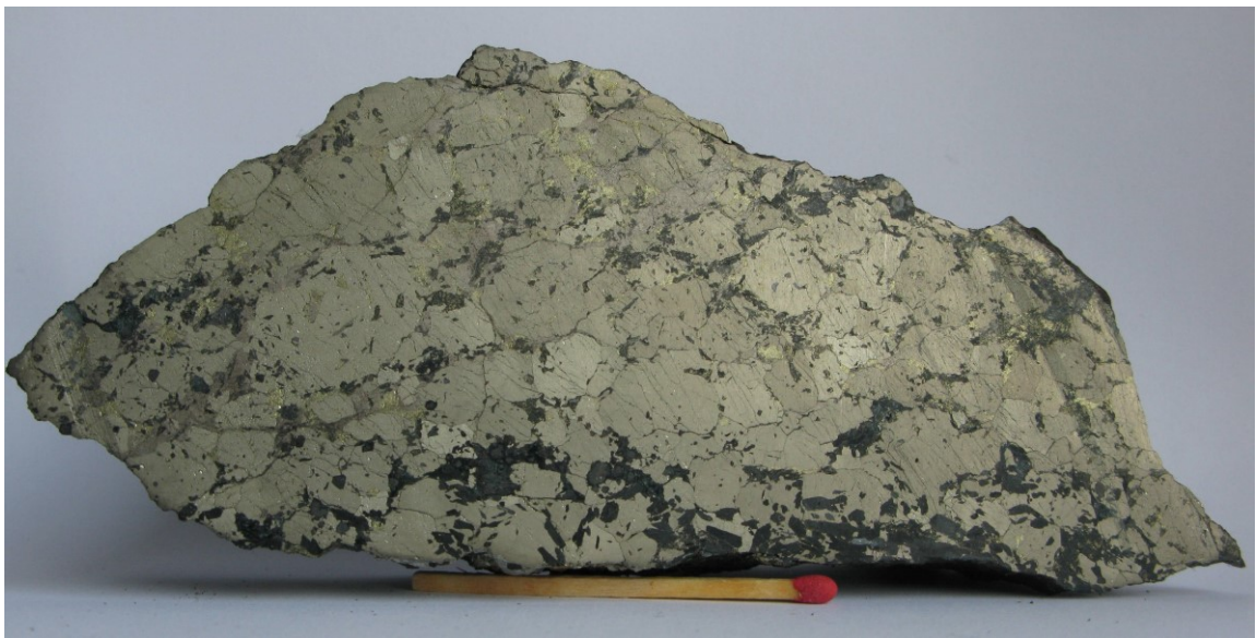
Fig. 2.12.3: Kisgruva. Massive pyrite (as recrystallized metablasts) and minor chalcopyrite and pyrrhotite. Not analyzed.
