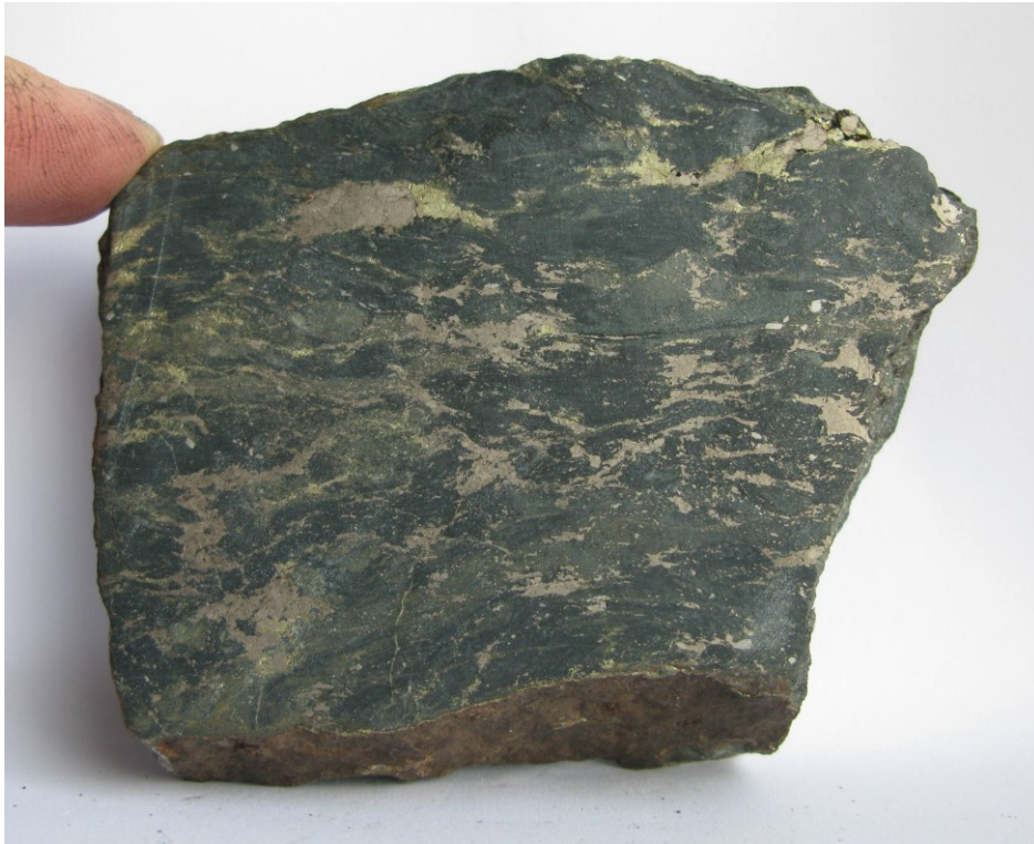
Fig. 2.13.2: Kopparvollane, sample 563358. Deformed chlorite-quartz schist with pyrrhotite, chalcopyrite and traces of arsenopyrite and magnetite.
