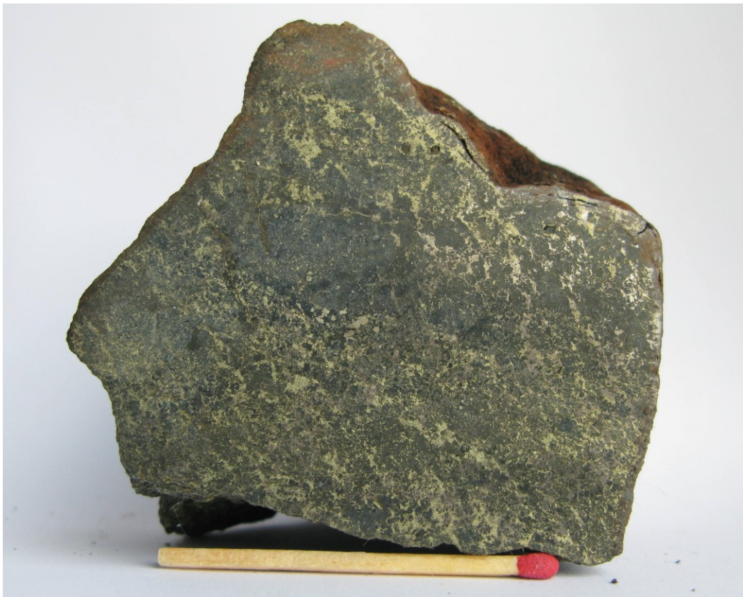
Fig. 2.16.2: Ore dump, sample 563359. Intensely deformed chalcopyrite and minor pyrite, pyrrhotite and sphalerite in quartz matrix.
