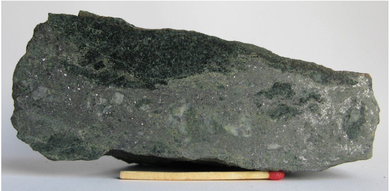
Fig. 2.7.4: Gunhildskås 1, sample 563365. Chloritized metabasalt above ore breccia of quartz and chlorite clasts and magnetite, galena and sphalerite.
