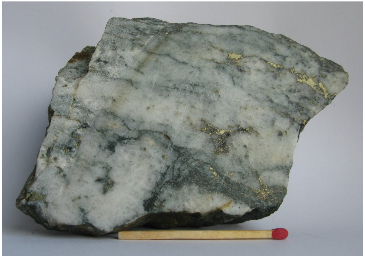
Fig. 2.7.5: Gunhildskås 1, sample 563366. Finegrained quartz with bands of chlorite and tourmaline. Chalcopyrite and traces of magnetite occur as fracture filling. This sample also has minor galena and sphalerite but not in this section.
