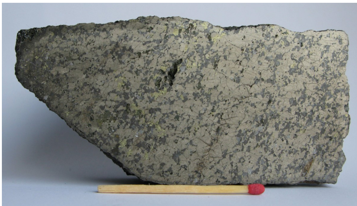
Fig. 2.11.2: Grøslø, sample 563354. Massive pyrrhotite with sphalerite, chalcopyrite and minor pyrite.
