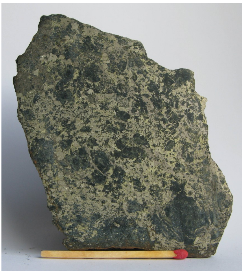
Fig. 2.15.2: Gotts Vermagt W, sample 563360. Deformed chalcopyrite, pyrite and pyrrhotite. The silicate phase is chlorite.
