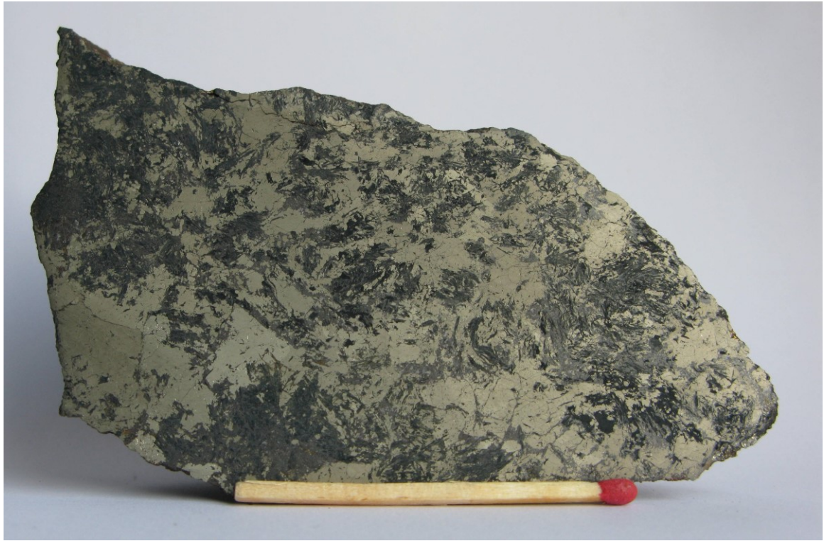
Fig. 2.17.2: Bergsgruva, sample 563362. Massive pyrite with sphalerite and minor chalcopyrite. Silicate is needle shaped amphibole.
