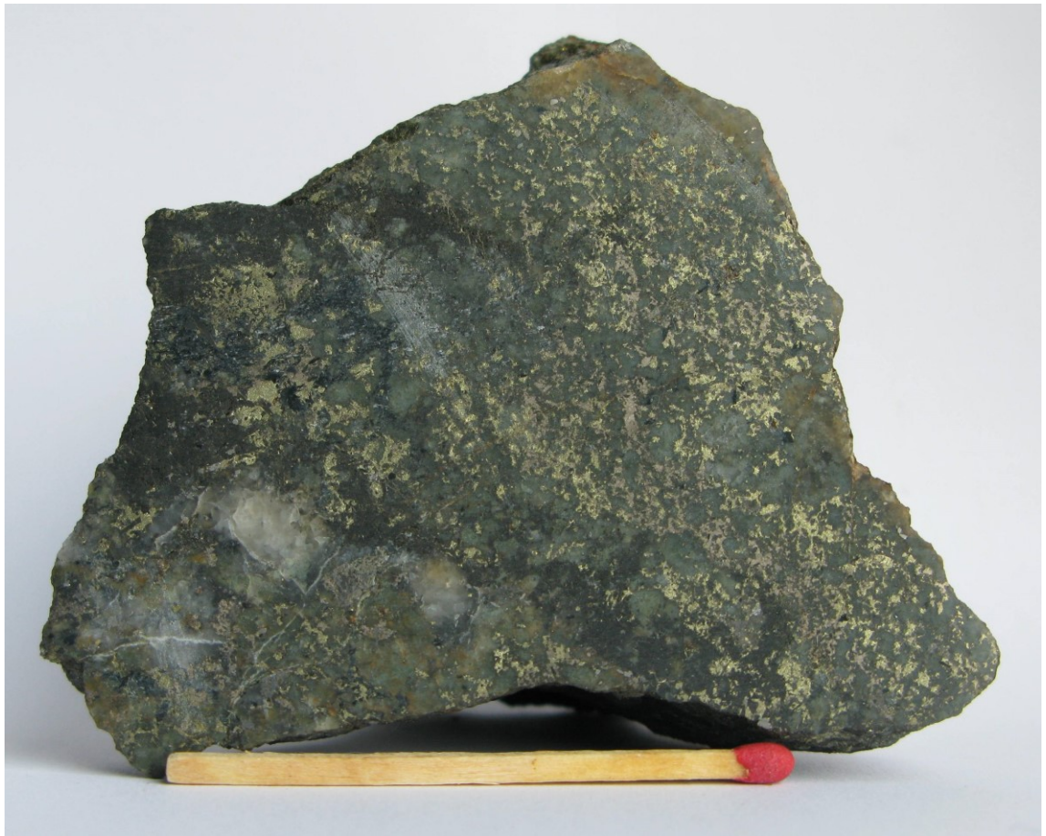
Fig. 2.1.2: Skyttemyr, sample 563330. Quartz and calc-silicates with chalcopyrite, sphalerite, pyrrhotite and löllingite and/or arsenopyrite.
