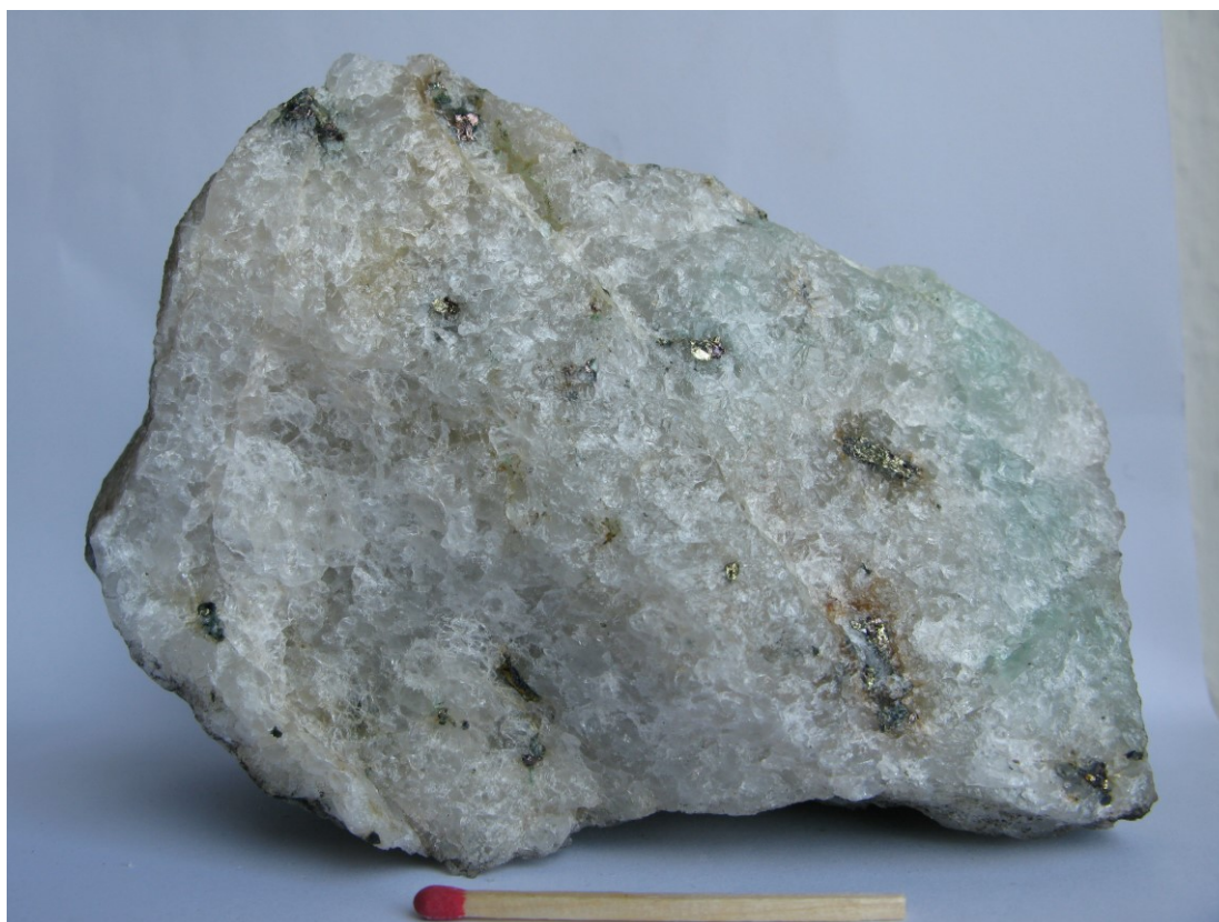
Fig. 2.10.2: Øvrestul 1. Specimen equal to sample 563350. Medium-grained quartz with disseminated chalcopyrite and bornite.
