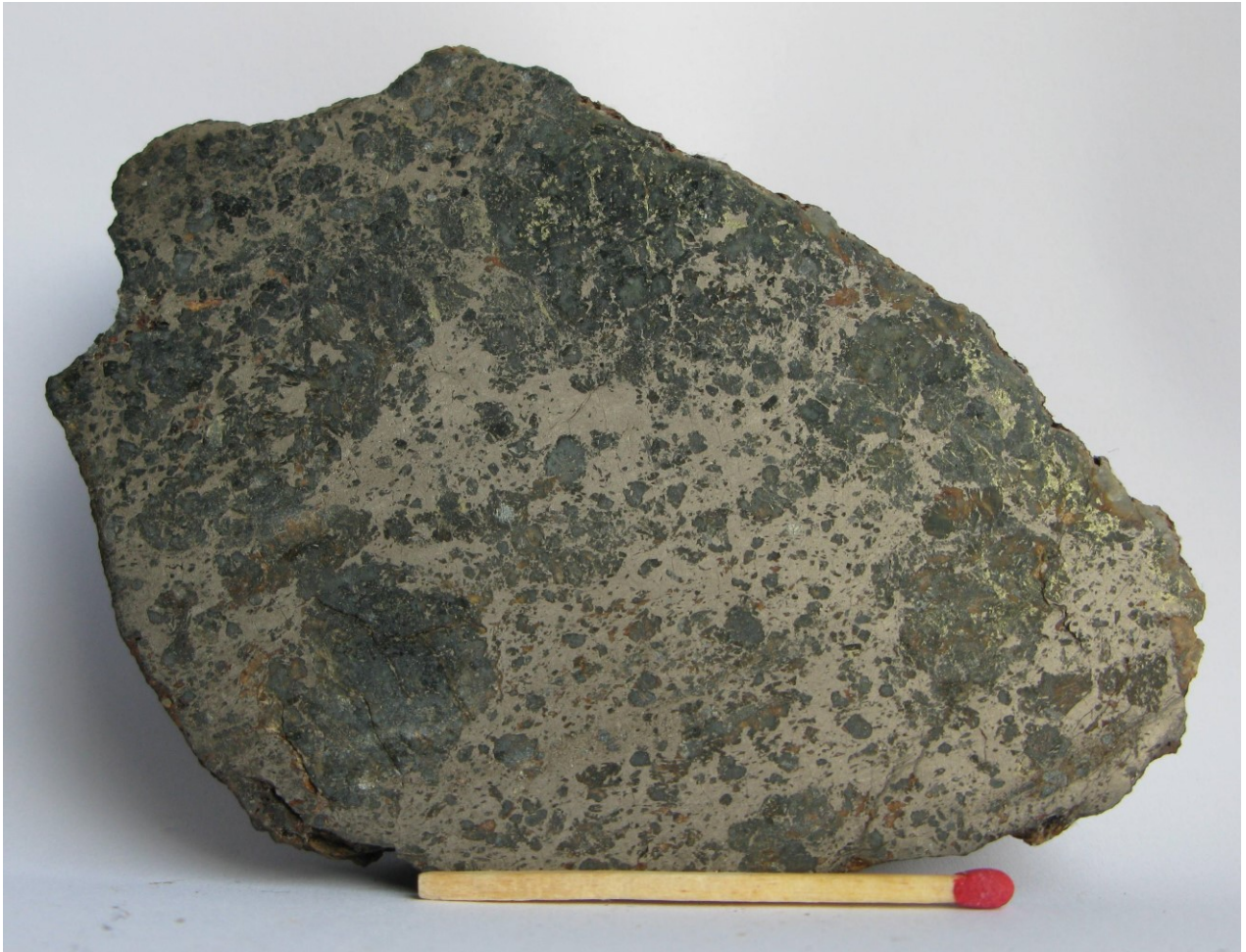
Fig. 2.3.2: Bøylestad, sample 563334. Pyrrhotite with rounded quartz and calc-silicate clasts. Only traces of chalcopyrite which mostly occurs as fracture-filling in silicate clasts.
