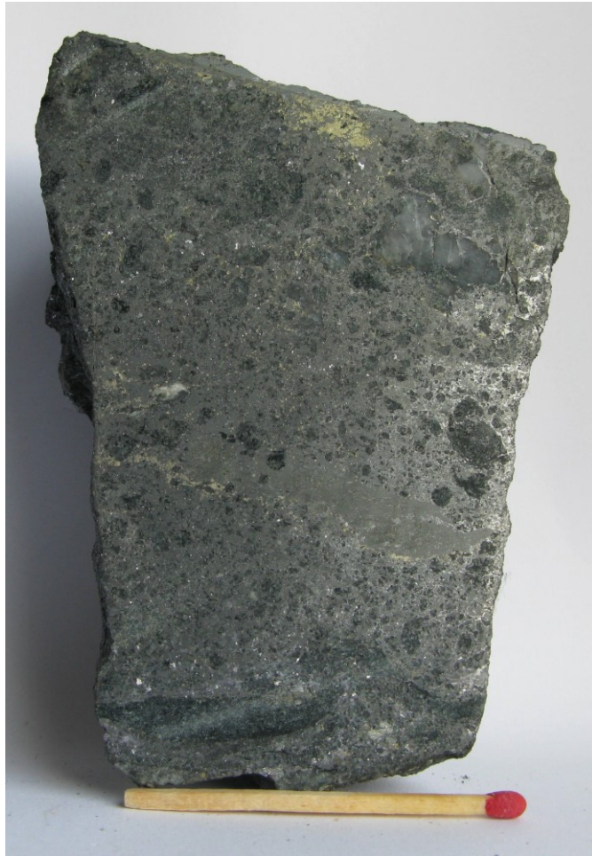
Fig. 2.6.2: Skolteberg, sample 563340. Fine-grained ore breccia with galena, sphalerite and minor chalcopyrite and magnetite. Rounded clasts (ball texture) are quartz and chloritized metabasalt.
