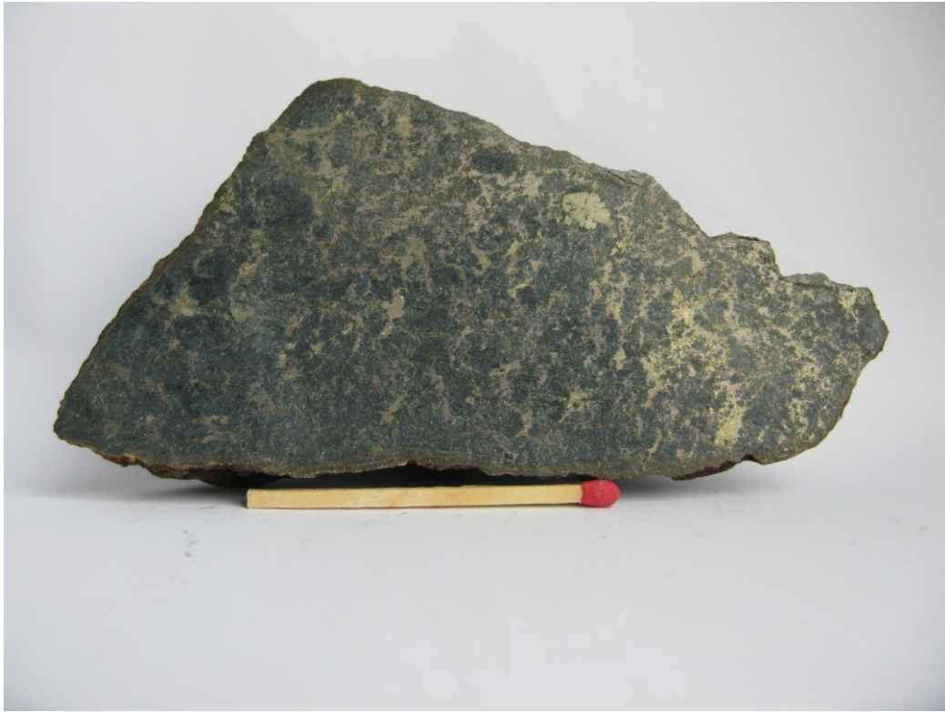
Fig. 2.14.2: Verlorne Sohn, sample 563356. Semimassive pyrrhotite & chalcopyrite in quartz. Also minor pyrite.
