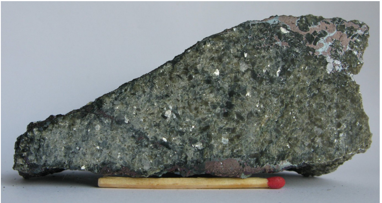
Fig. 2.9.2: Grusen. Completely sericitized arenite with chalcosite (bluish) replacing bornite (brown). Not analyzed.
