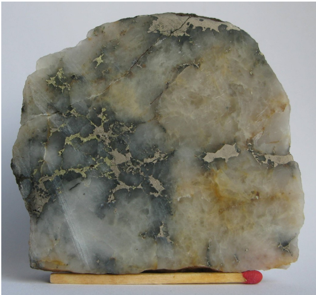
Fig. 2.4.3: Espelandsmyr, sample 563336. Quartz with pyrrhotite, chalcopyrite and traces of galena and sphalerite as fracture-filling.
