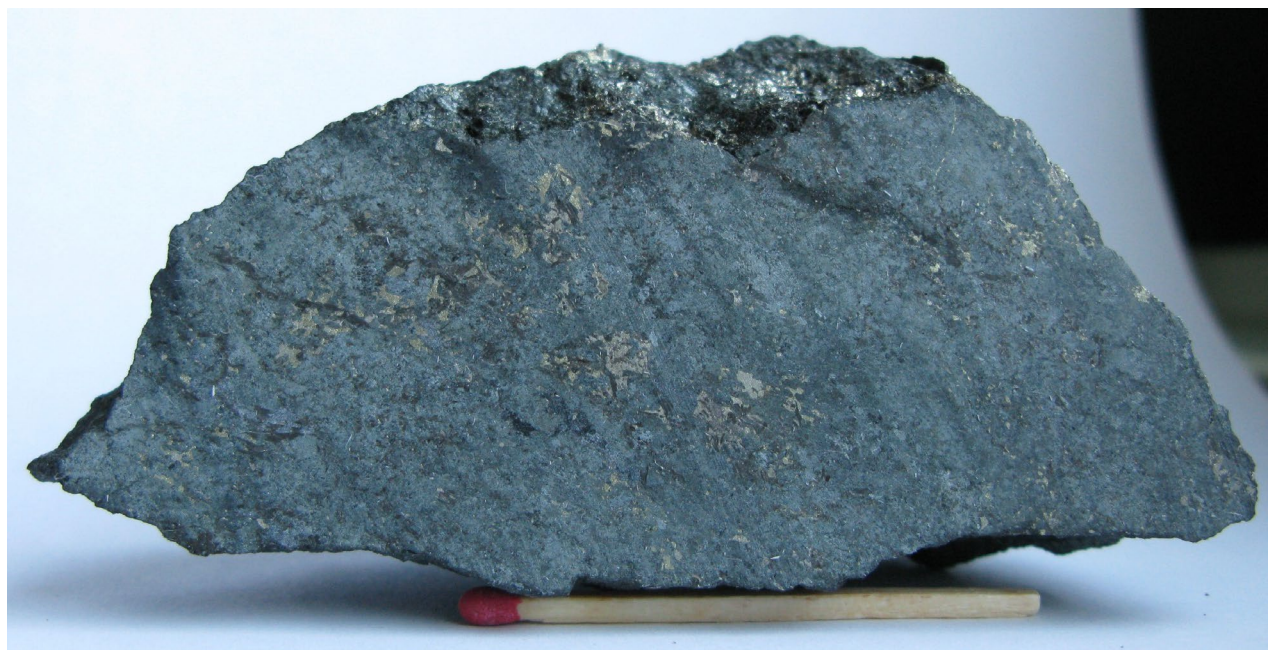
Figure 2.30A: Eknes, amphibolite with disseminated pyrrhotite, chalcopyrite and pentlandite.
