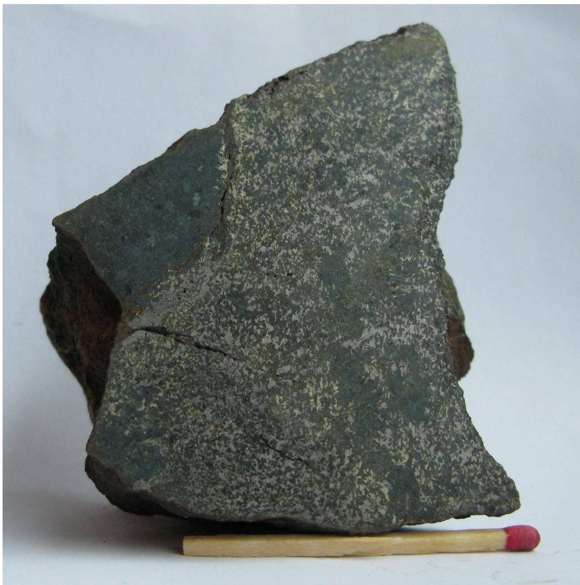
Figure 2.35A: Øvredal, semi-massive pyrrhotite>chalcopyrite in serpentinite.
