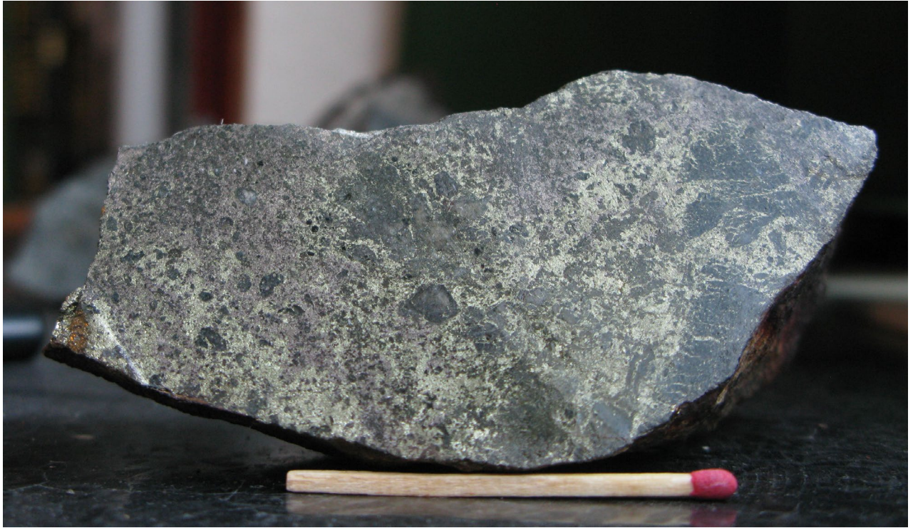
Figure 2.9A: Søyset, sample 563239, ball-texture, chalcopyrite>pyrrhotite with rounded/cataclastic fragments of host-rock.
