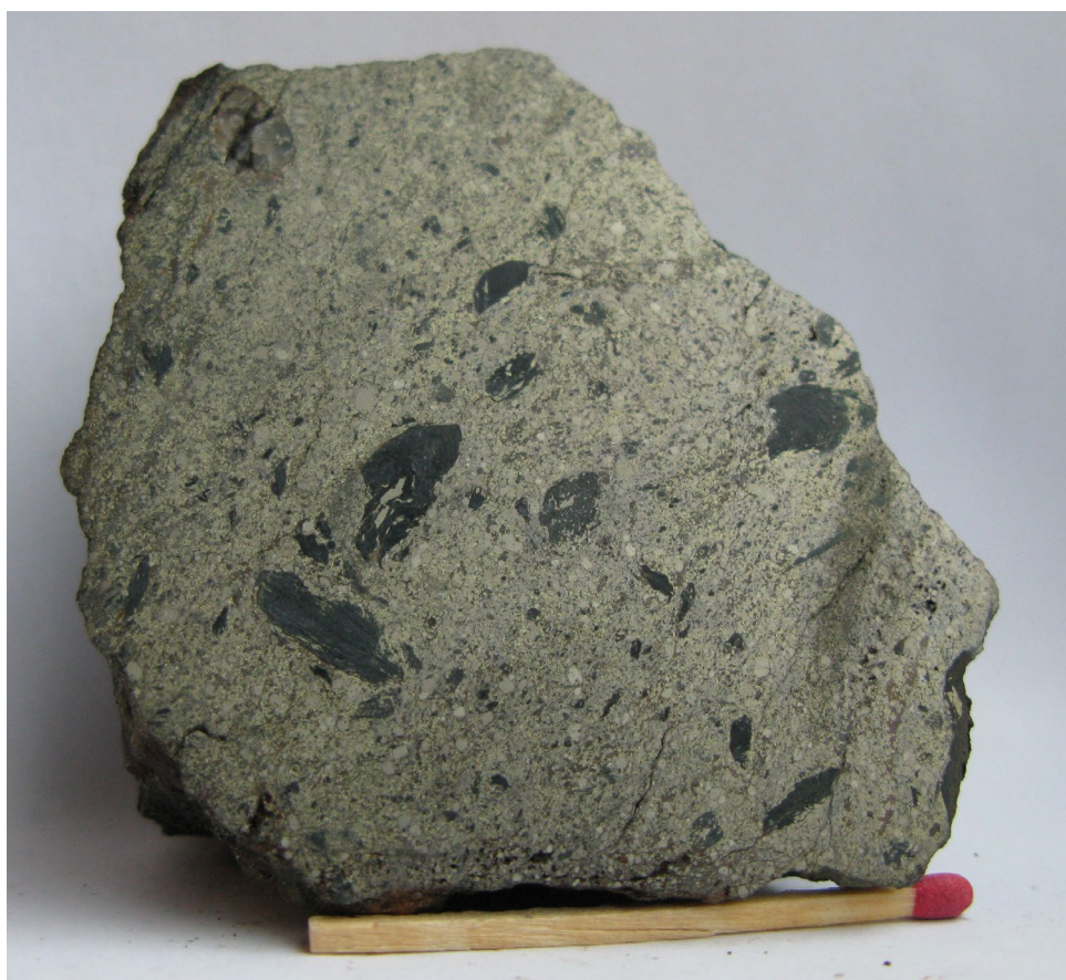
Figure 2.16B: Vågene, ball-texture, pyrite>chalcopyrite+sphalerite with rounded fragments of host-rock.
