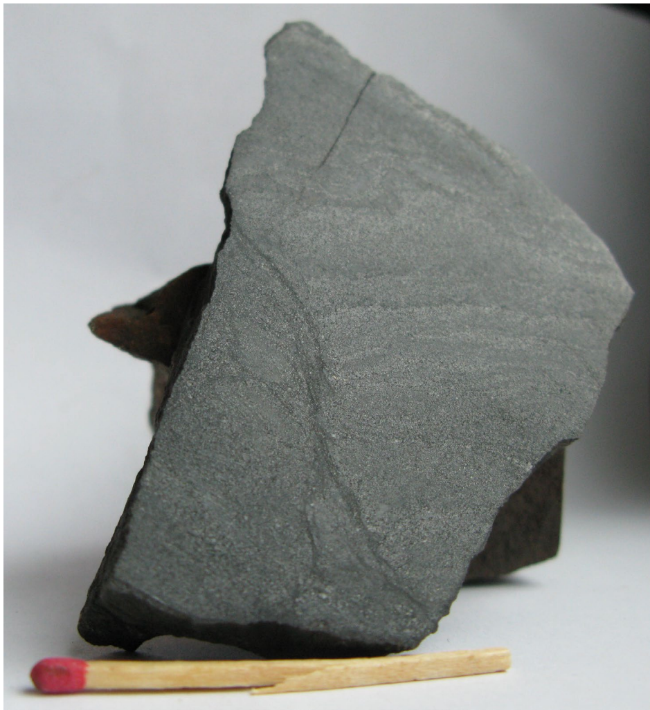
Figure 2.18B: Gjerdvika, banded, fine-grained magnetite and quartz (metamorphosed ochre?).
