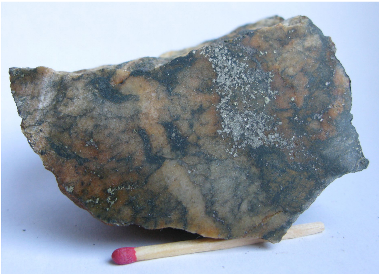
Figure 2.1A: Flatskarvåsen, rusty quartz with uneven dissemination of pyrite>chalcopyrite.
