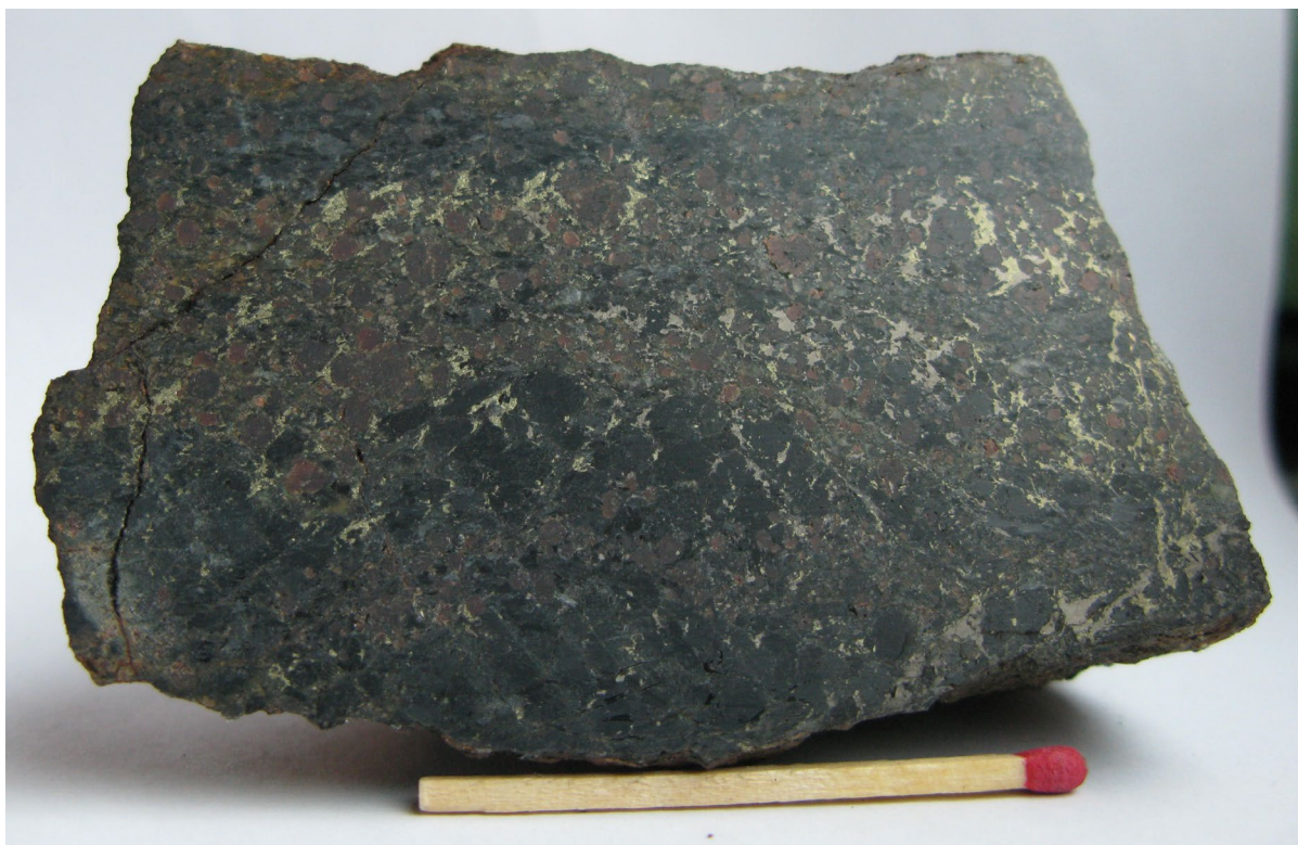
Figure 2.6D: Averøy A11, garnet-amphibole gneiss with chalcopyrite & pyrrhotite.
