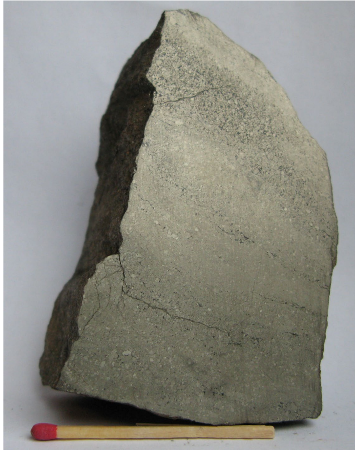
Figure 2.17A: Grimeli, fine-grained and weakly banded massive pyrite with chalcopyrite > sphalerite.
