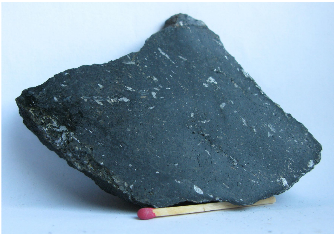
Figure 2.40A: Fuglavatnet, amphibolite with disseminated arsenopyrite.
