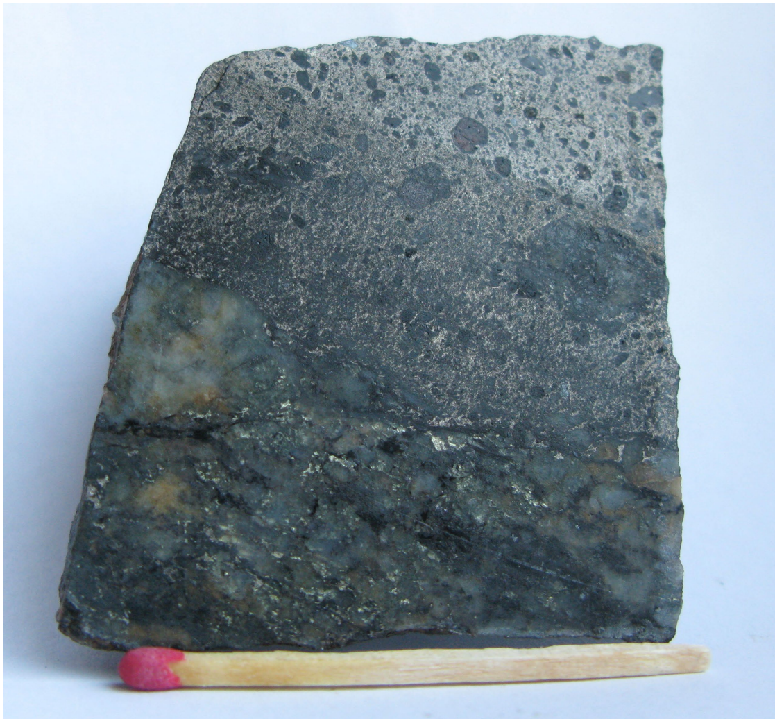
Figure 2.6B: Averøy A5, upper part of photo: ball-texture, pyrrhotite with rounded amphibole.
