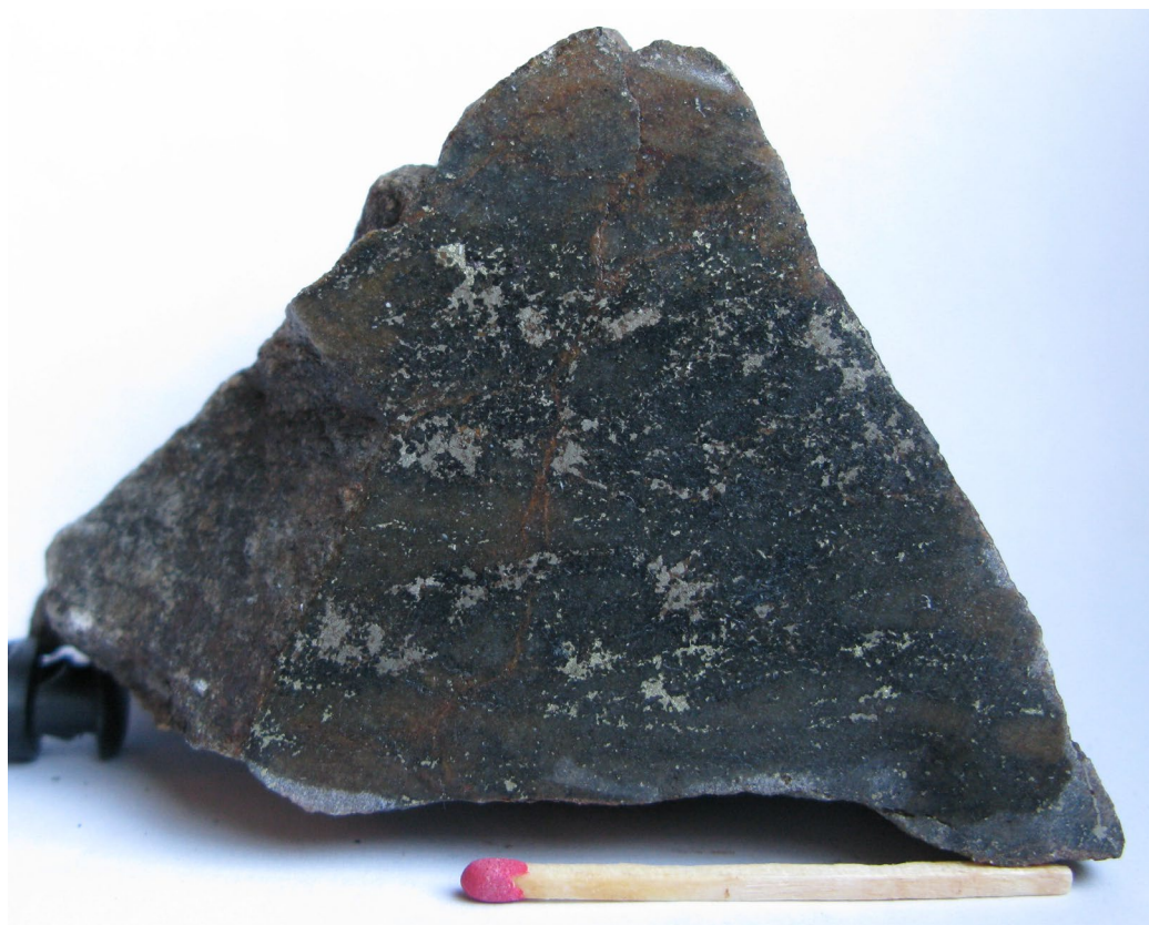
Figure 2.44A: Garborg, pyrrhotite+chalcopyrite in quartz matrix (there are far more sulfide-rich specimens but they are very weathered).
