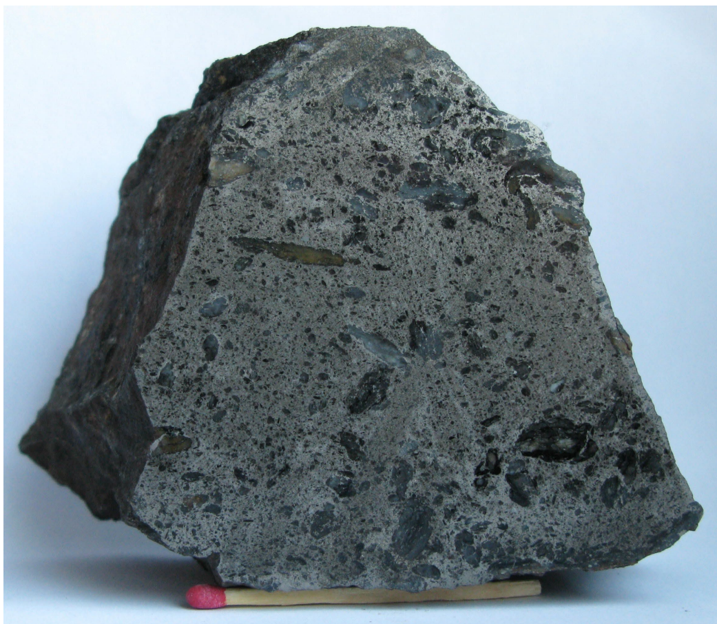
Figure 2.8C: Bevre 2, ball-texture, pyrrhotite with rounded fragments of host-rock and quartz.
