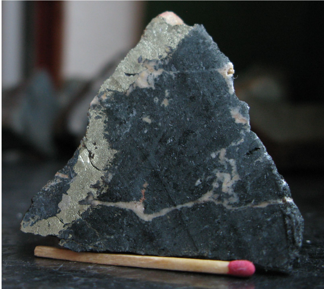
Figure 2.26A: Velesvik, dolerite with chalcopyrite>pyrite-vein and K-feldspar-veinlets.
