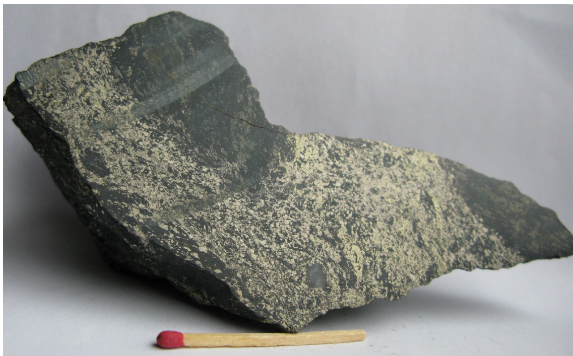
Figure 2.18C: chloritized basalt with pyrite>chalcopyrite.
