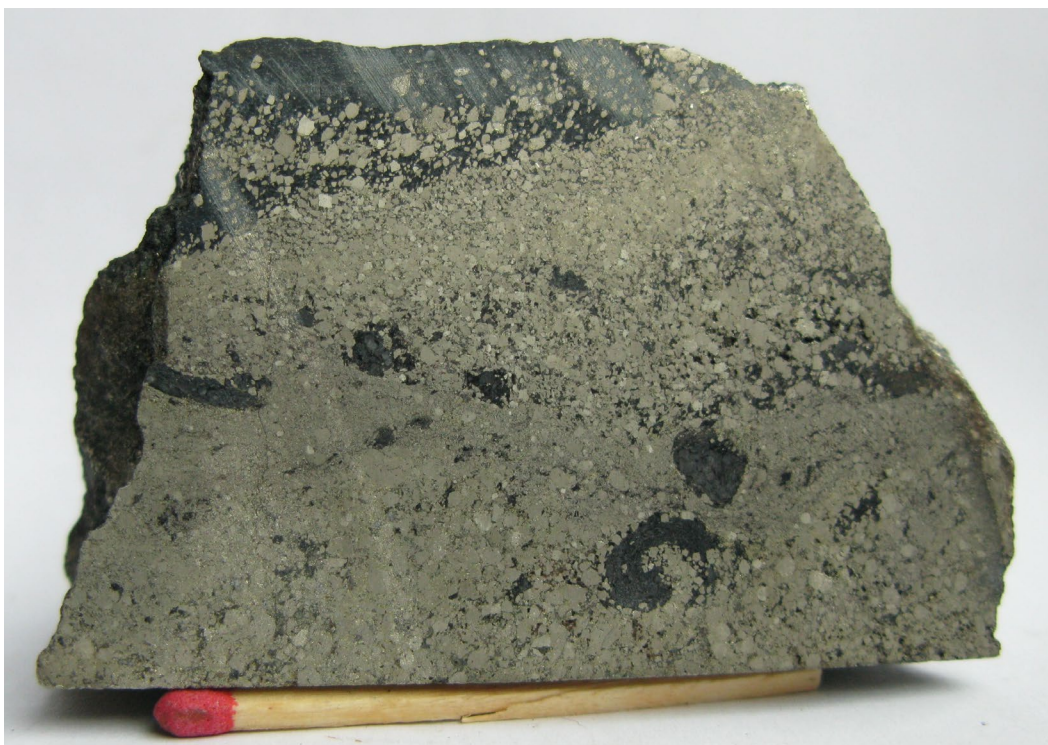
Figure 2.20B: Svanøy, very deformed, mostly fine-grained pyrite>chalcopyrite+sphalerite.
