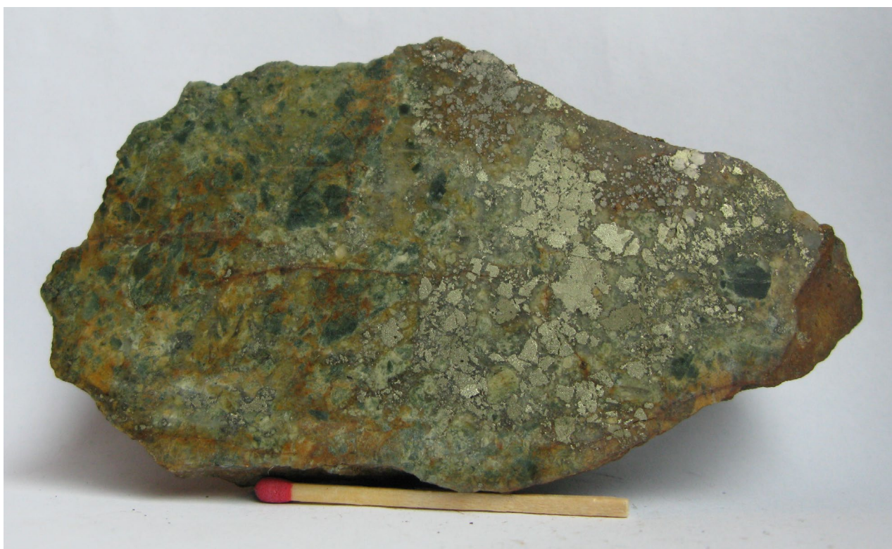
Figure 2.29A: Espetveit, brecciated anorthosite with plenty chalcopyrite and minor pyrite.
