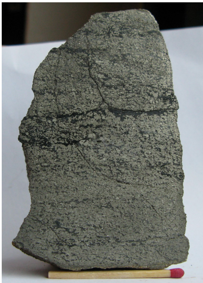
Figure 2.37B: Massive pyrite. Matrix is quartz but the dark layer may be chlorite.
