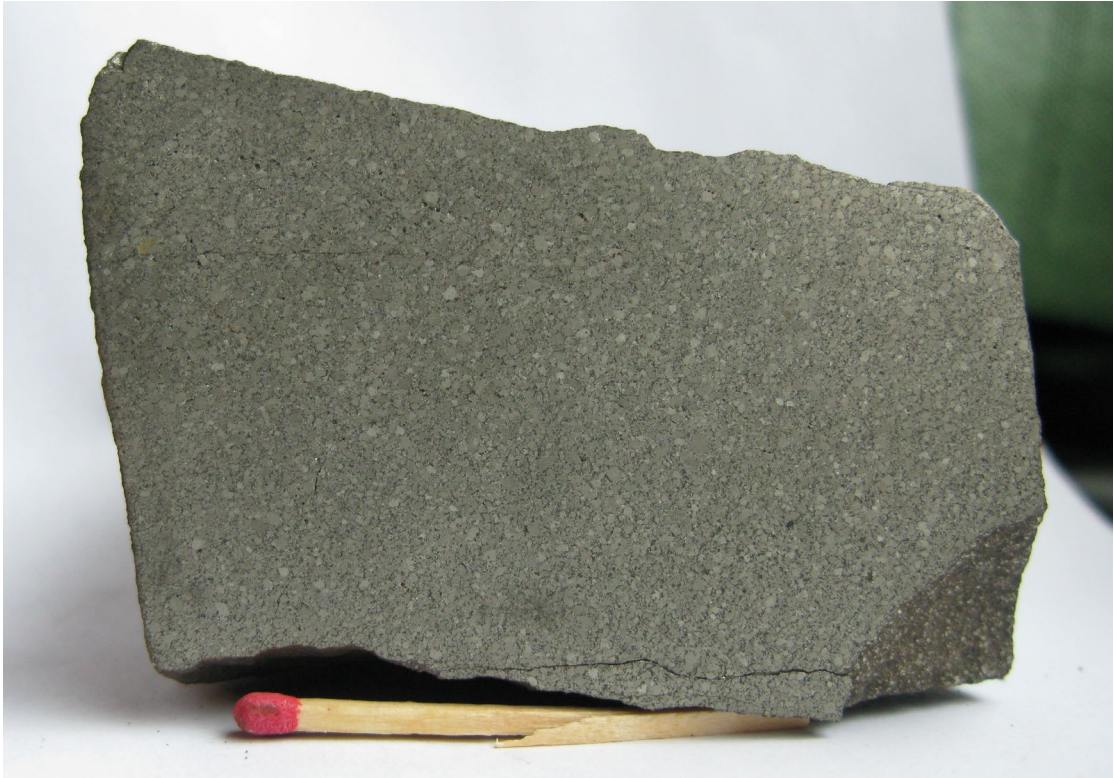
Figure 2.18A: Gjerdvika, massive pyrite with chalcopyrite and sphalerite.
