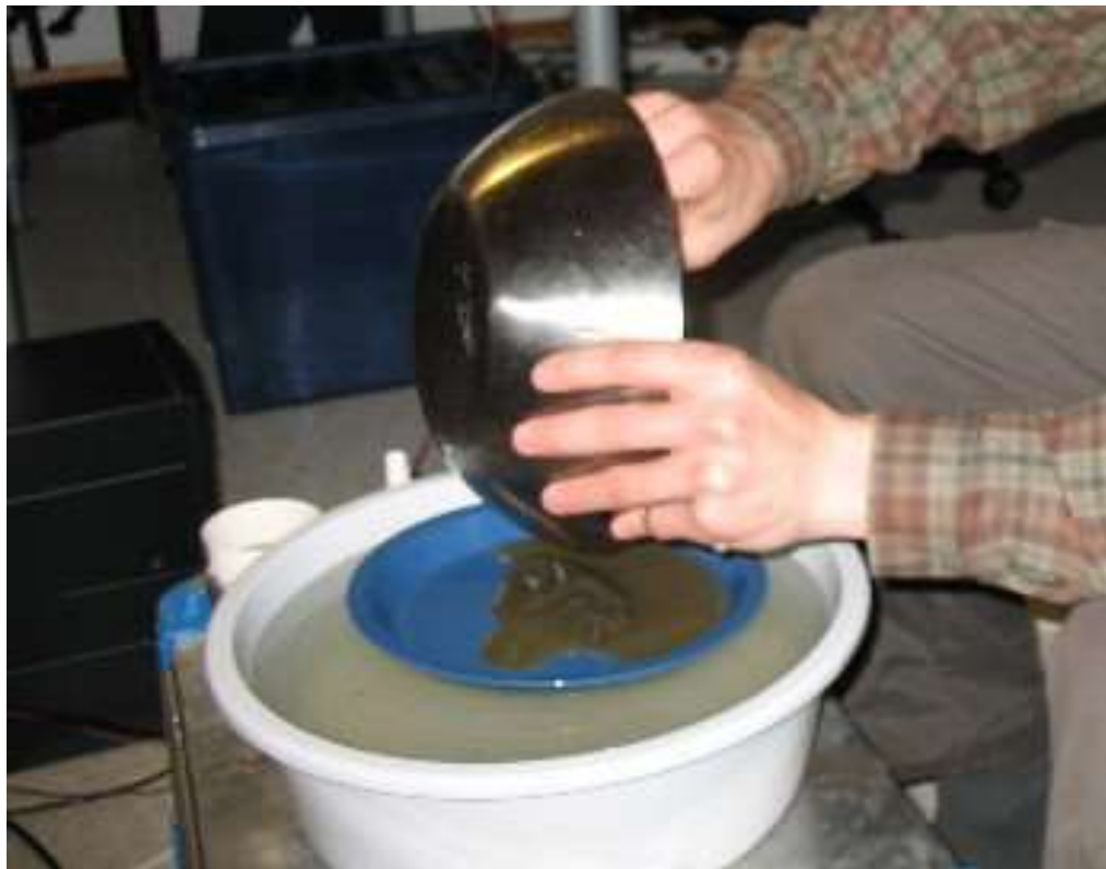
Figure 108 The sieved sample is washed in to the panning plate.
