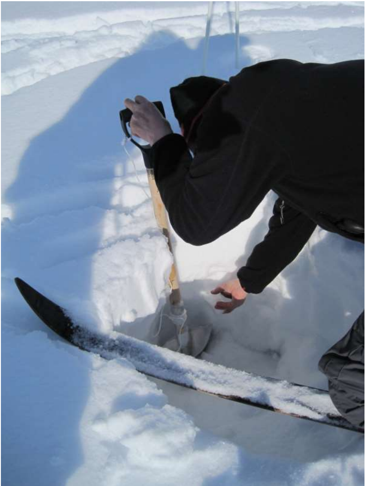
Figure 100 Juhani Ojala scooping the sample into the 120 ml container.
