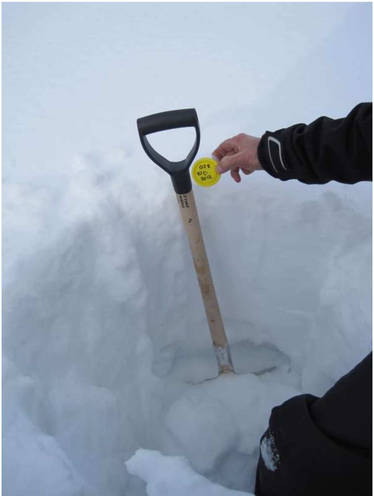
Figure 99 Typical sampling depth is about 45 cm above the snow-ground interface. At this level snow changed from coarse grained sugary snow at the bottom to fine grained snow on the top.
