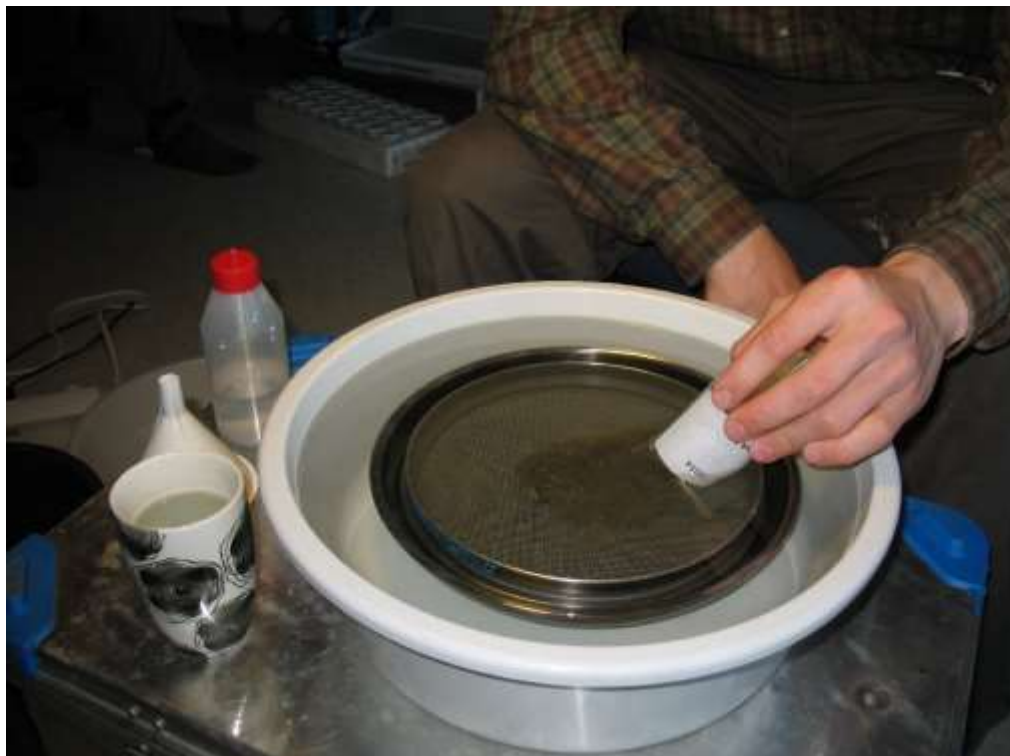
Figure 106 Pre-concentrated sample is sieved underwater using a 0.5 mm sieve.
