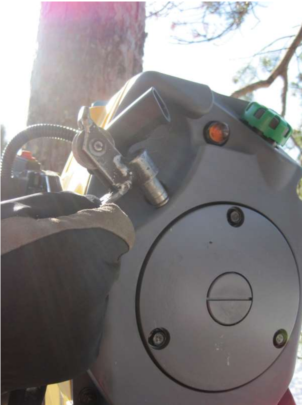
Figure 92 The starter rope modification part made by the Geological Survey of Finland.
