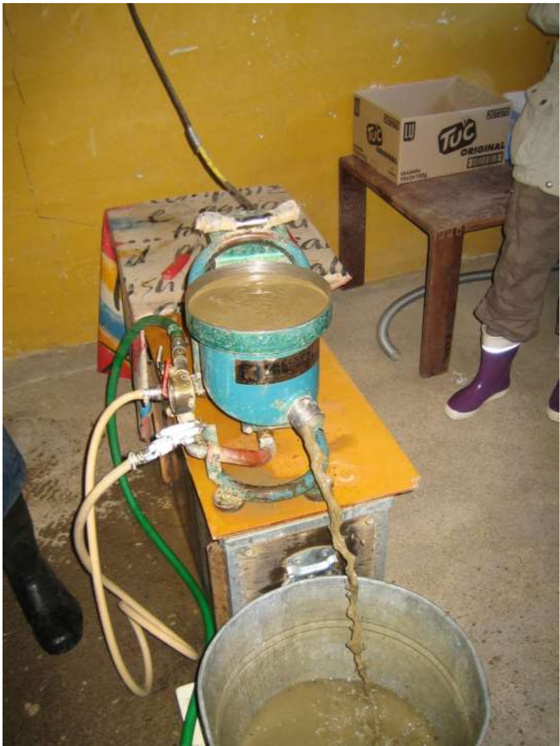
Figure 102 Slurry goes to the device through a metal funnel. Knelson working.
