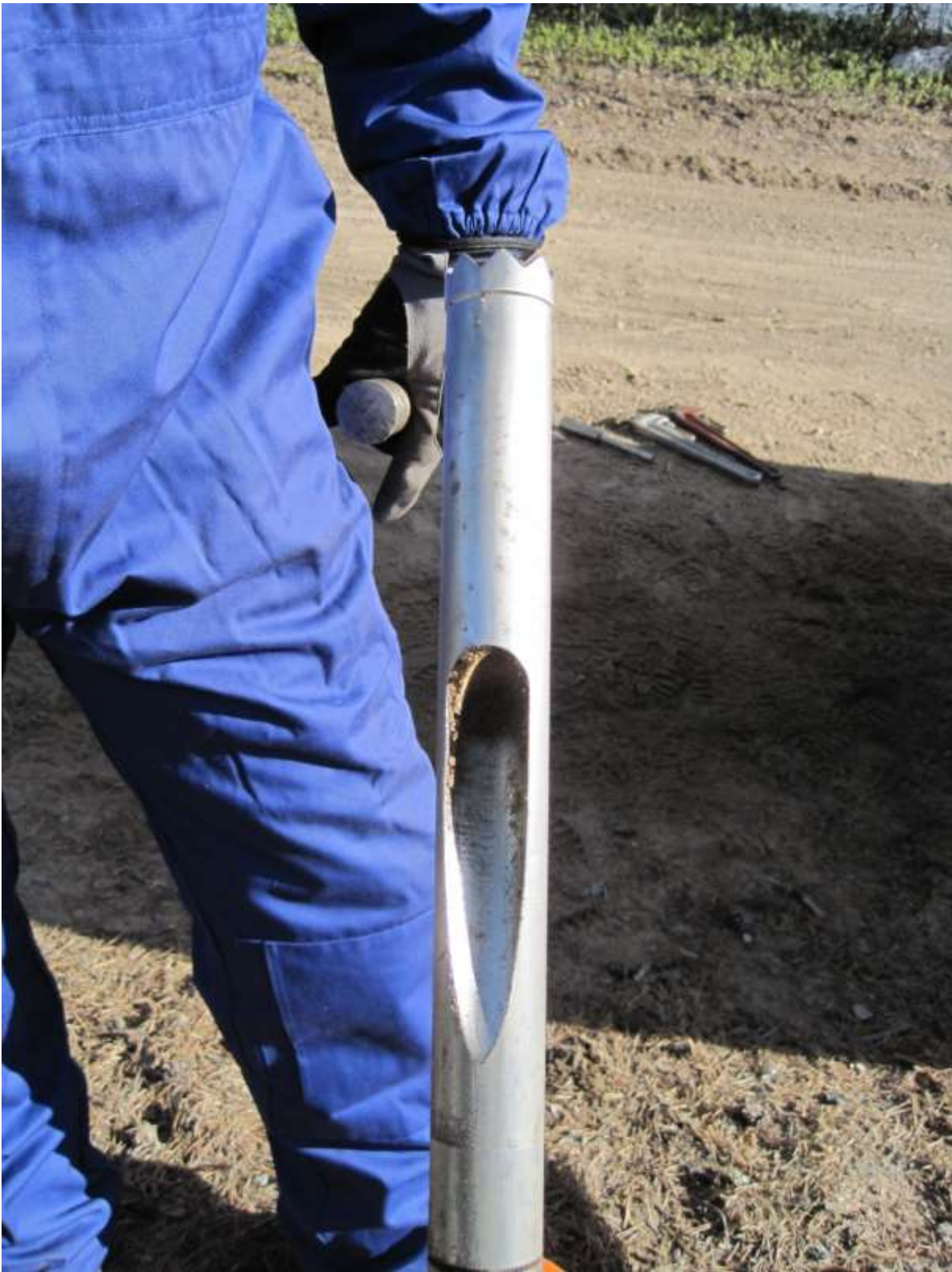
Figure 90 Sample is ready to be taken out with the steel stick.
