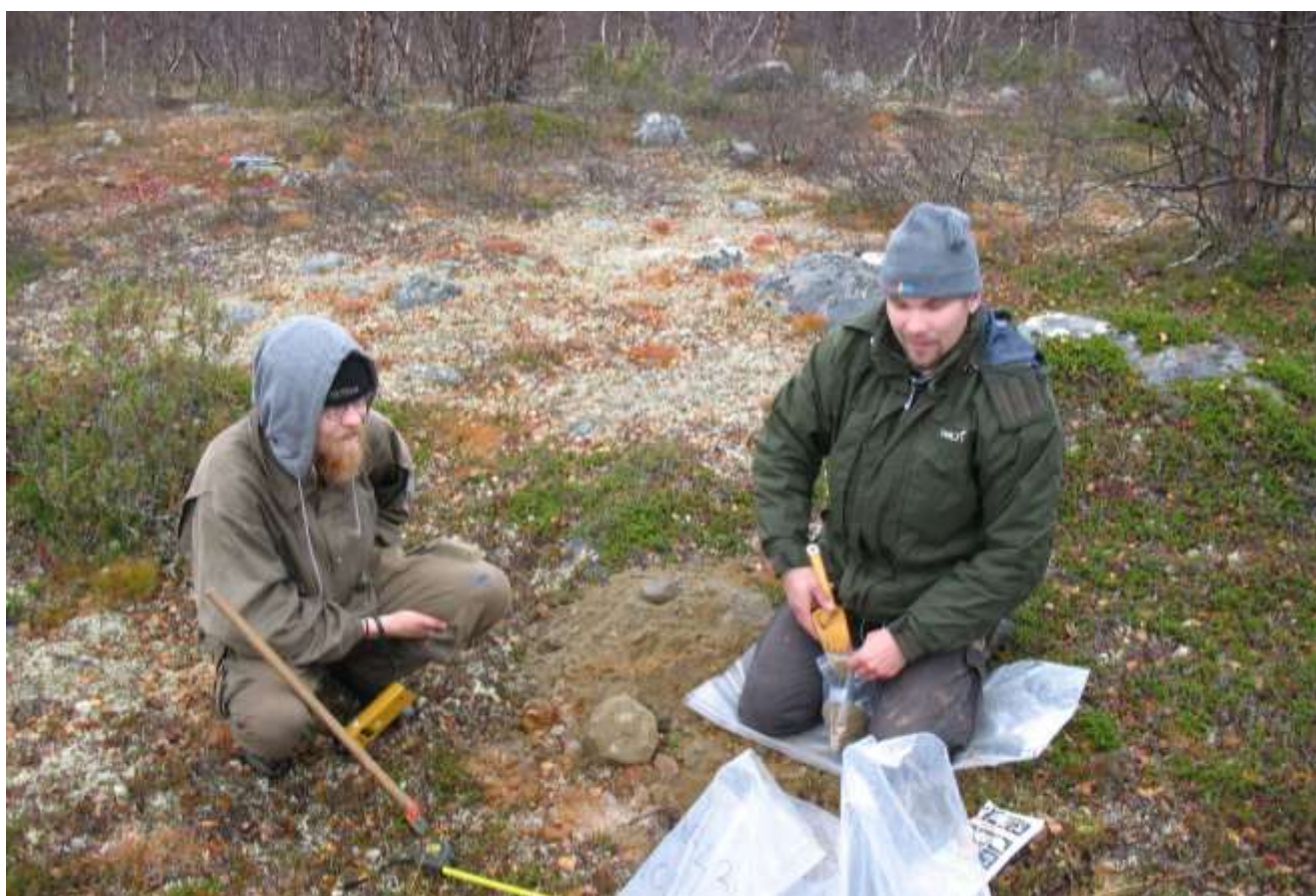
Figure 97 Sample is collected to a zip-lock bag.
