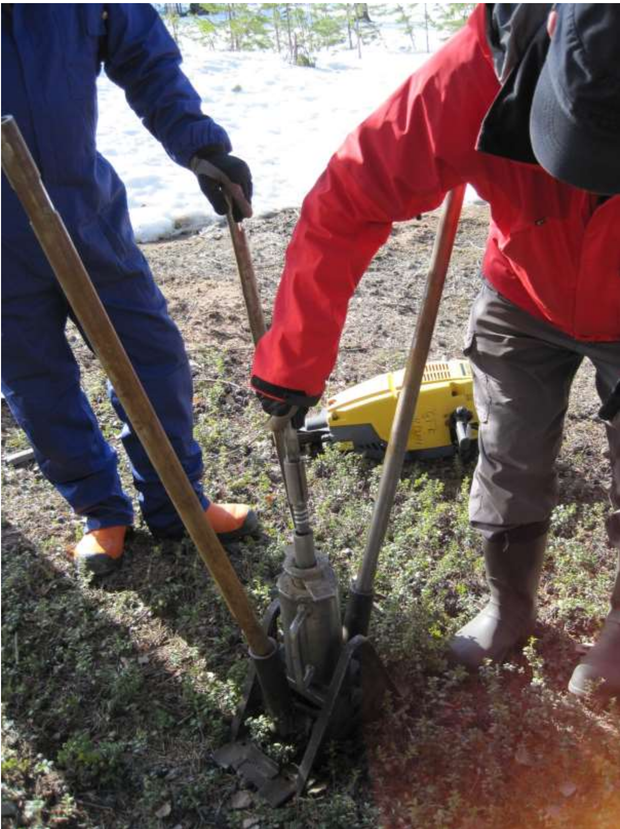
Figure 89 Rods are pulled out with a jack. The adapter is attached to the coupling before the last rod is pulled out. This will keep the coupling clean.
