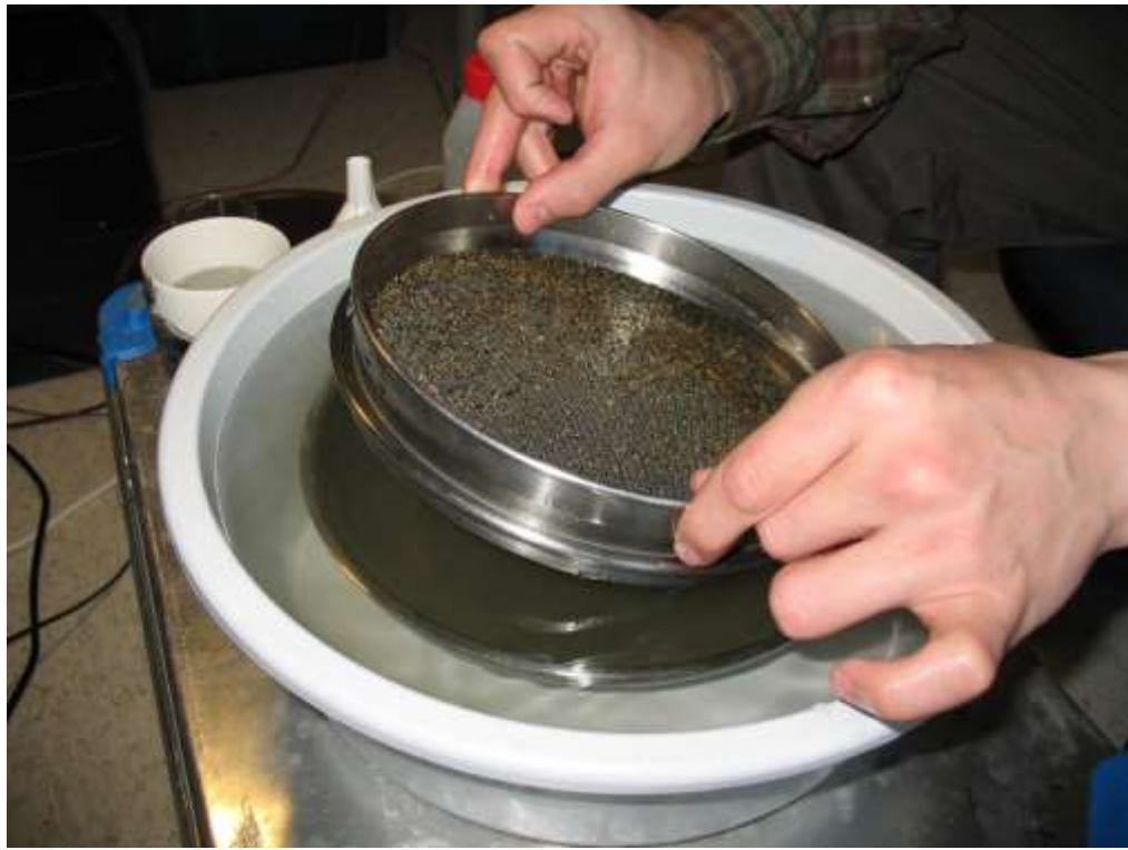
Figure 107 The 0.5-2 mm fraction is observed briefly for gold grains.
