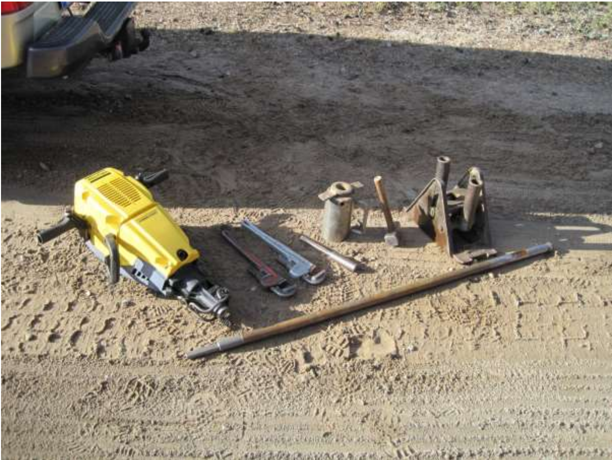
Figure 87 From left to right; Cobra Combi hammer drill, wrenches, stick to empty the sample chamber, rod holder, hammer and jack. Below; there is a rod with a tip sampler (flow through bit) and an adapter attached.
