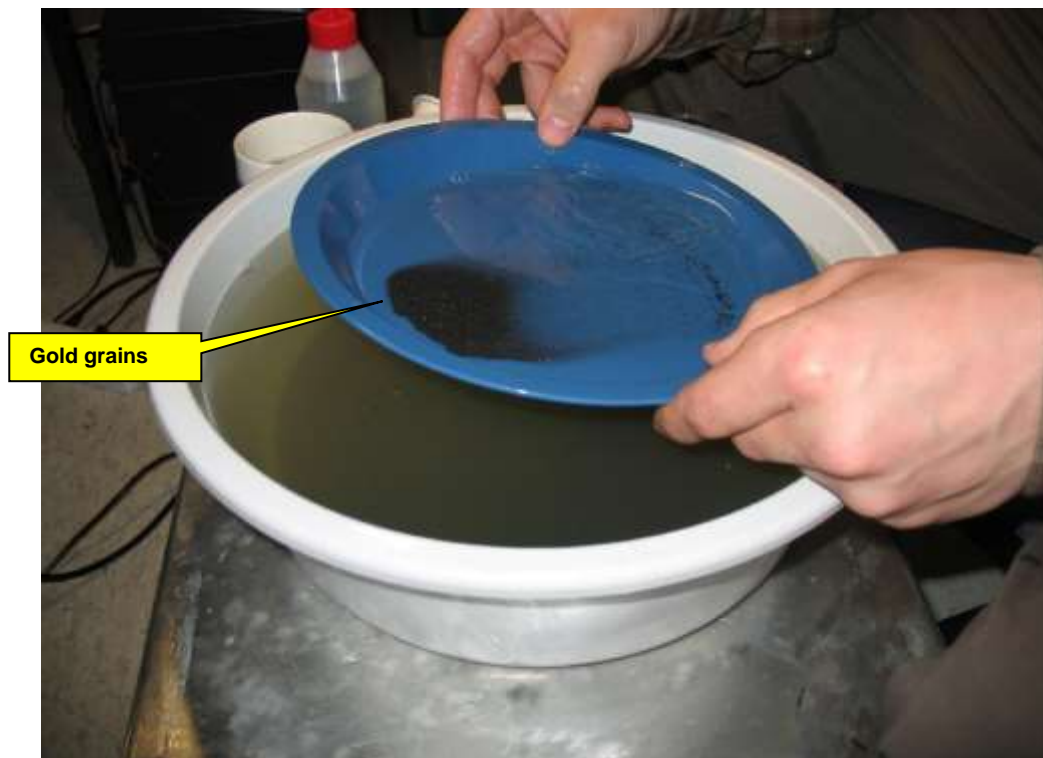
Figure 110 Sample is turned over. The gold grains are found from the tip of the “grain fan.”
