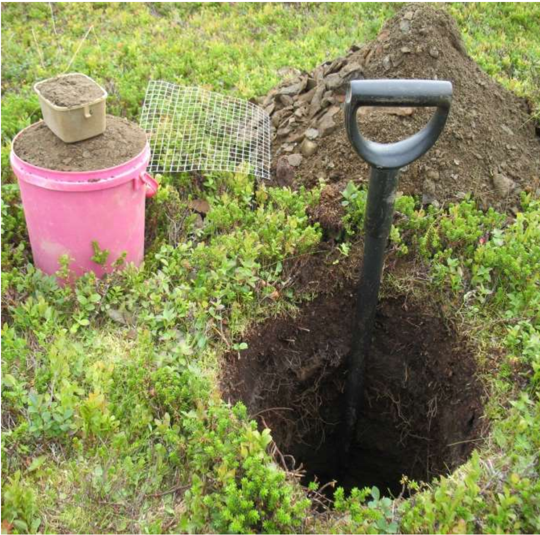
Figure 85 Heavy mineral (10-12 kg) and geochemical sample (~800 g) taken.
