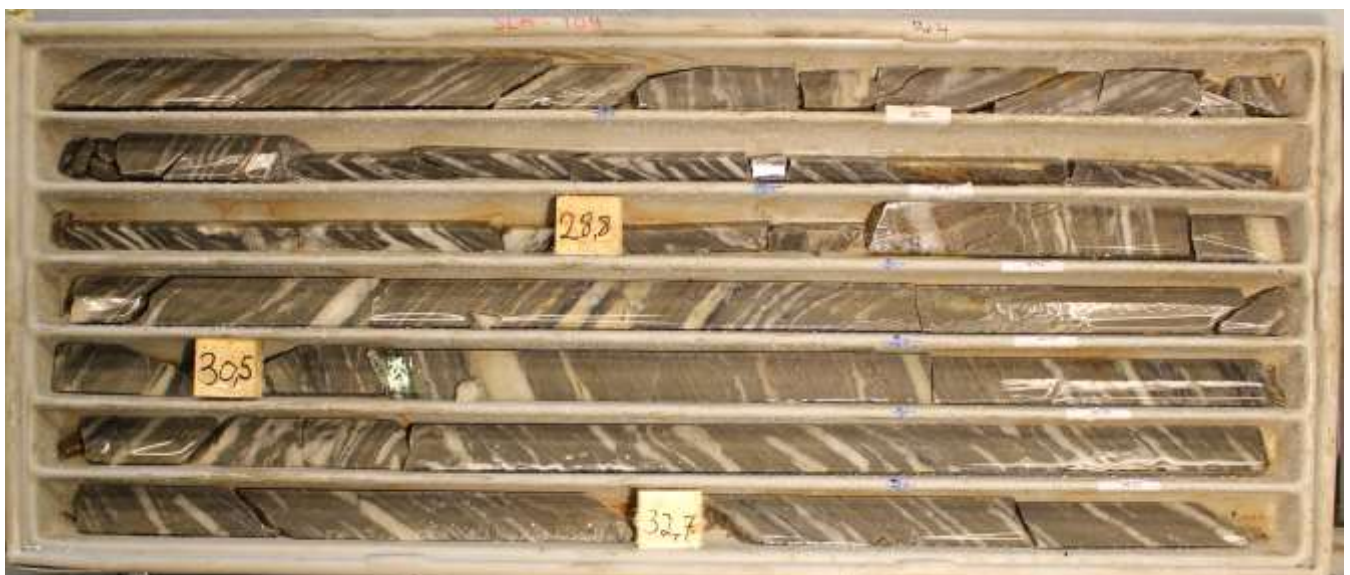
Figure 19 Photograph showing drill core of banded iron formation, highest value 1.46 g/t Au is the sample interval 28-29 m.
