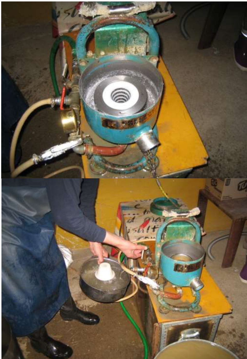
Figure 104 Sample is flushed from the cone in to a kettle.
