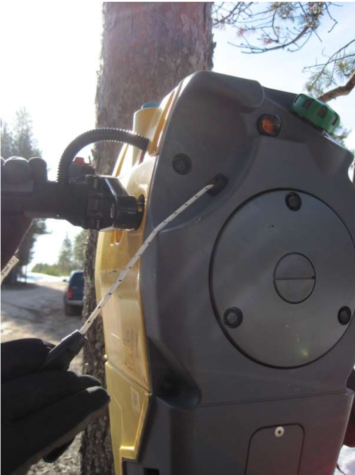
Figure 93 If not modified, the starter rope will eventually wear out and break, because of the pulling angle.
