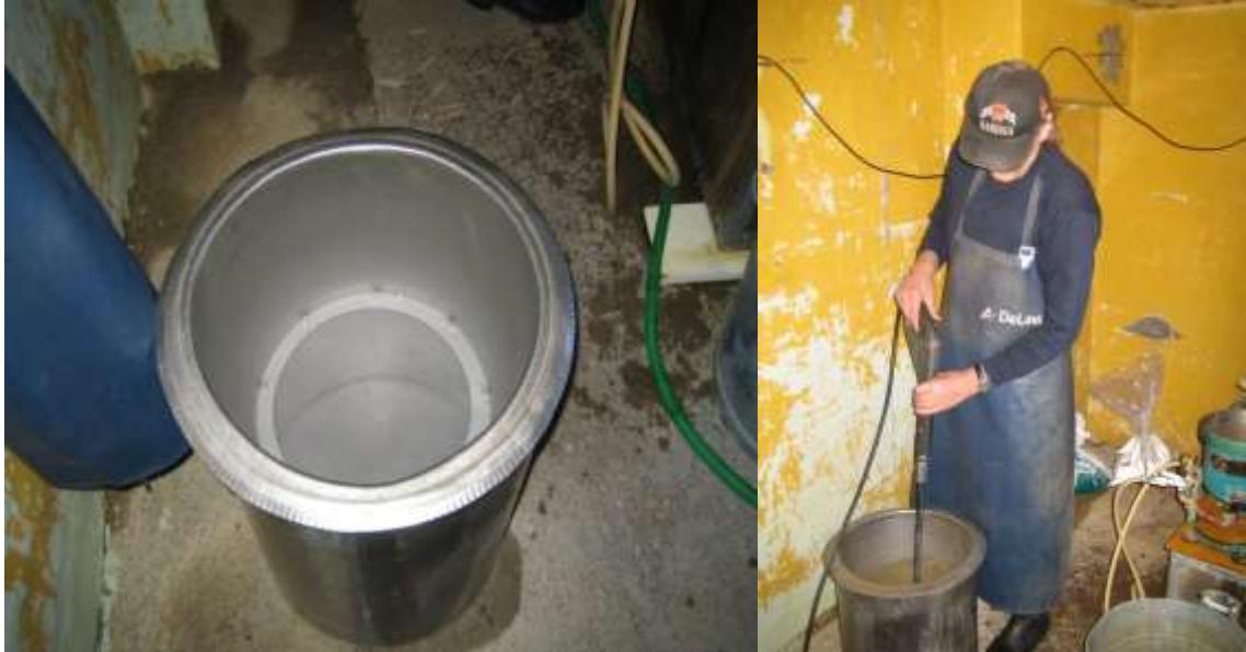
Figure 101 Heavy mineral sample is wet sieved in to a big container.
