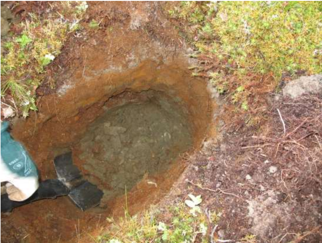
Figure 84 Colour of the overburden changes when the unaltered till is reached.
