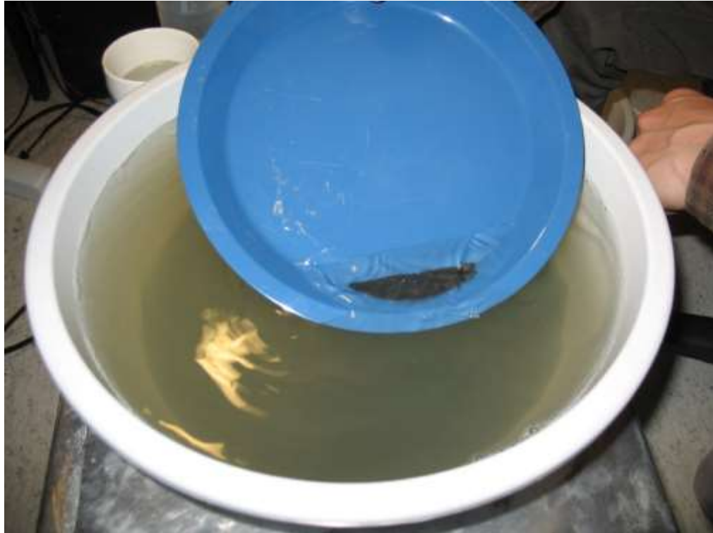
Figure 109 Sample is almost ready to be turned over. Gold grains are in the bottom.
