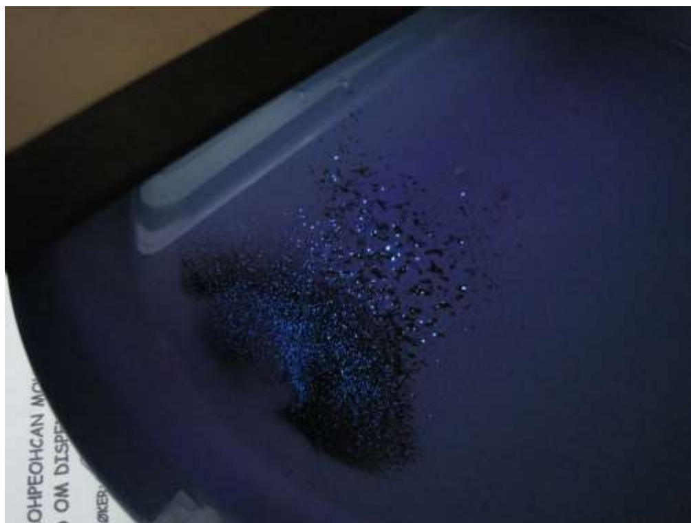
Figure 113 Scheelite grains under shortwave UV. Grain size 0.03-0.9 mm.
