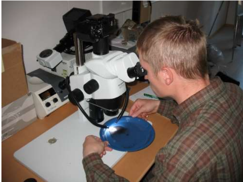
Figure 111 Counting and observation of the grains with a stereomicroscope.
