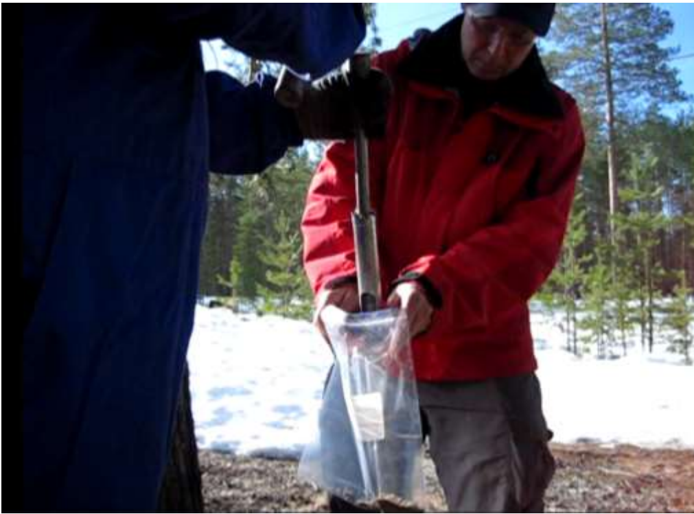
Figure 91 Sample is taken out with the steel stick with slight hammering.
